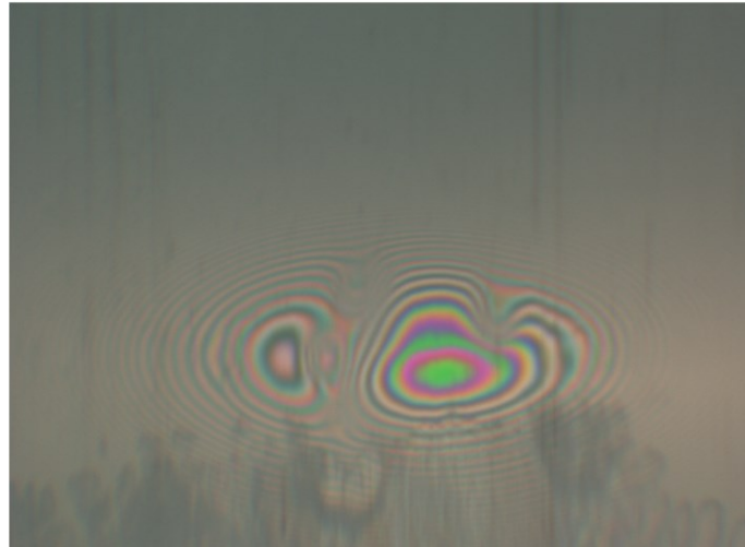
Figure 7.16: Image of the rolling contact at a ring speed of 0.076 m/s, lubricated by the PU 220 grease.
