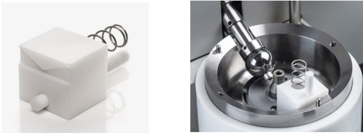
Figure 3.2: a) PCS Instruments grease scoop. b) The grease scoop in position in the MTM, seated on the disc specimen [168].
