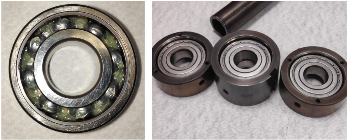
Figure 3.7: a) A bearing prepared with ~1.4 g of grease. b) The three assembled bearing housings making up a single test unit ready for assembly onto the drive shaft.
