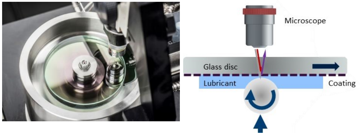
Figure 3.4: a) Disc specimen in pot, with microscope in position [175]. b) Diagram of EHD function.
