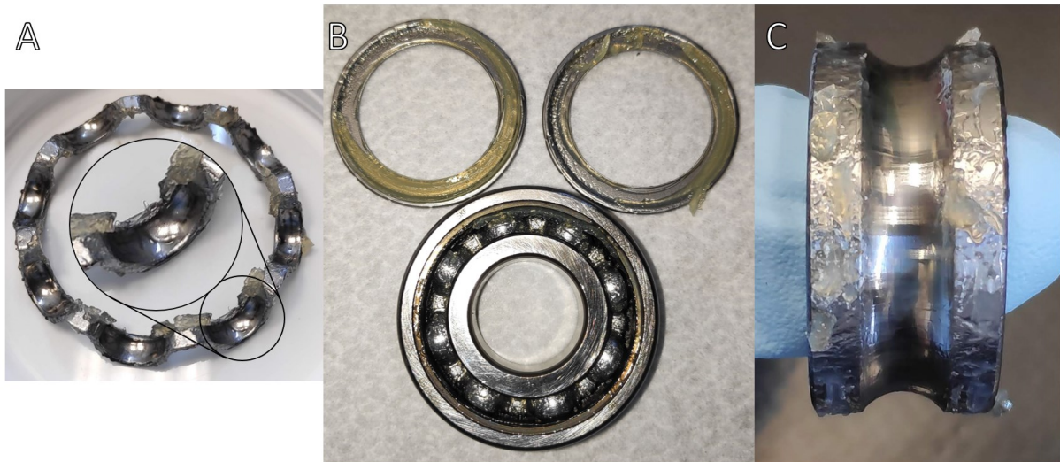
Figure 4.9: A partially dismantled bearing run at 5,000 RPM, lubricated with CaXB 100 grease. A) one half of the cage, showing oil-rich semi-fluid lubricant within the cage pockets, and grease that appears much 'drier' on the other parts of the cage. B) Bearing after removal of the shields, showing variability in the distribution of grease on the shields, both circumferentially and between the two sides. C) The inner race, showing very thin, fluid, films within the raceway.
