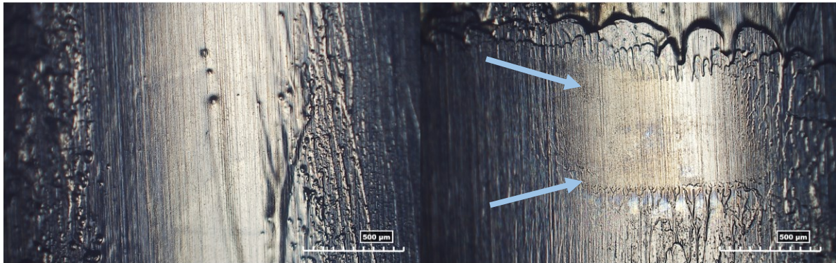
Figure 4.19: Images of the PU 220 bearing raceway.
