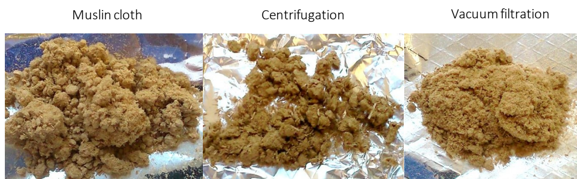
Figure II-40. Images of clean pulp after washing using 16 equivalents of ethanol by a) muslin cloth, b) centrifugation and c) vacuum filtration. Miscanthus pulp recovered after pretreatment of Miscanthus at 120 °C for 6 hours at 0.5L scale using stirring at 20 wt% loading.
