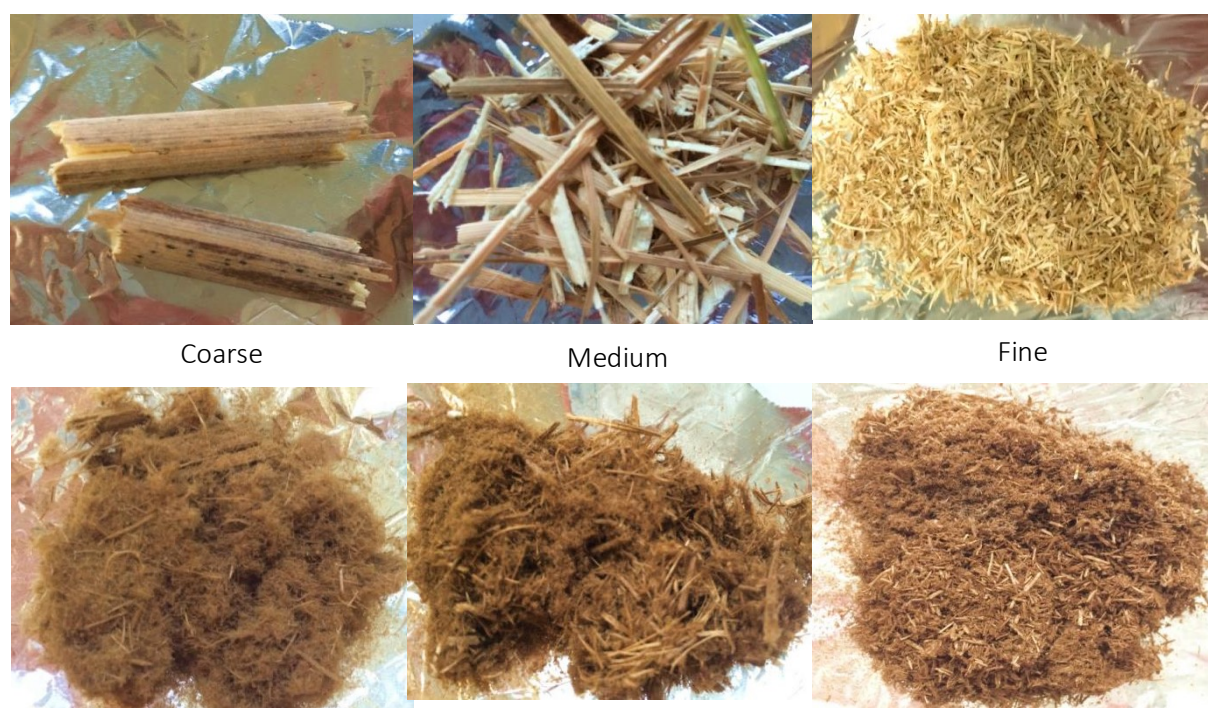
Figure II-32. Photographs of (a) untreated biomass and (b) recovered pulps after pretreatment of Miscanthus with [TEA][HSO 4 ] at 120 °C for 6 hours at bench scale using a biomass loading of 20 wt%.
