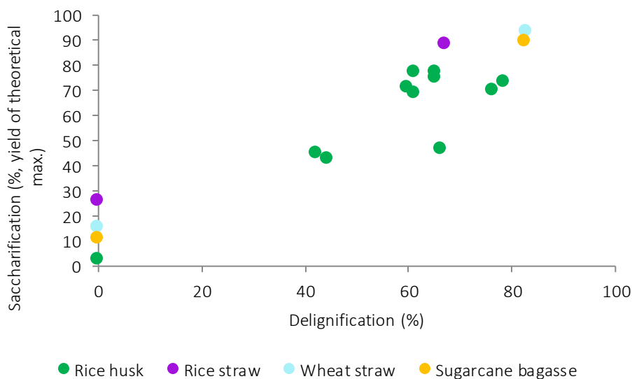
Figure S0-1. Saccharification yields vs. delignification of pulps before and after pretreatment of rice husk, rice straw, wheat straw and depithed sugarcane bagasse under various conditions.
