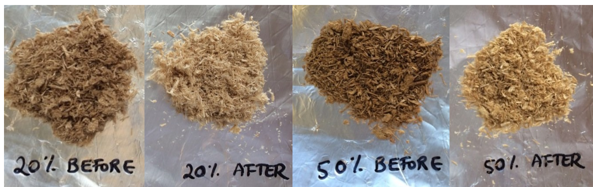
Figure II-29. Pretreated Miscanthus pulps obtained before and after washing with DMSO for biomass loadings of 20 wt% and 50 wt%.
