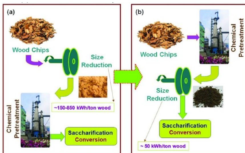
Figure I-11. Schematic diagram showing the approach for mechanical wood size-reduction operation from (a) pre- to (b) post-chemical pretreatment to reduce energy consumption. Reproduced from Zhu et al. 344
