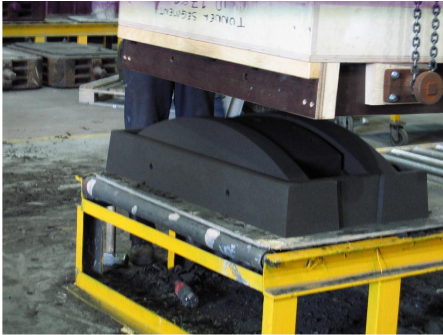
Figure 4-3. Bottom part of sand mould.
