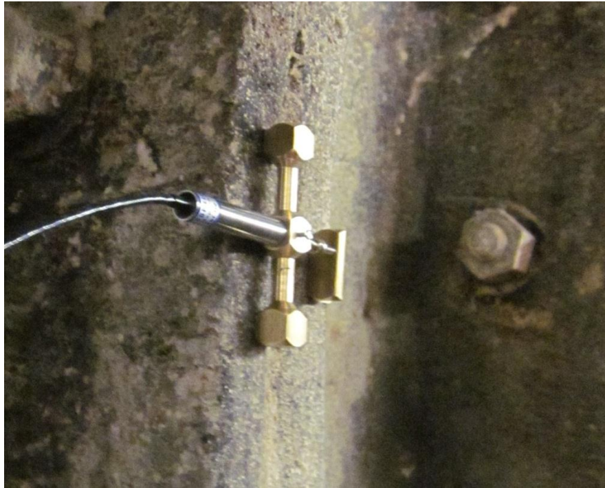
Figure 3-6. LVDT displacement transducer in metal holder.
