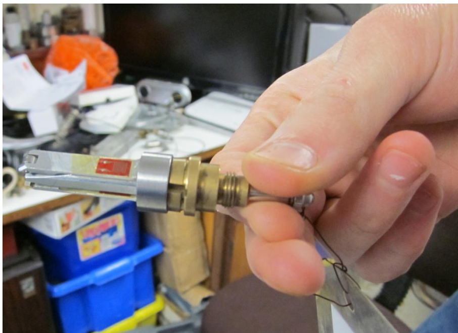
Figure 6-16. The inside of a strain gauged displacement transducer, with hand holding onto plunger rod.
