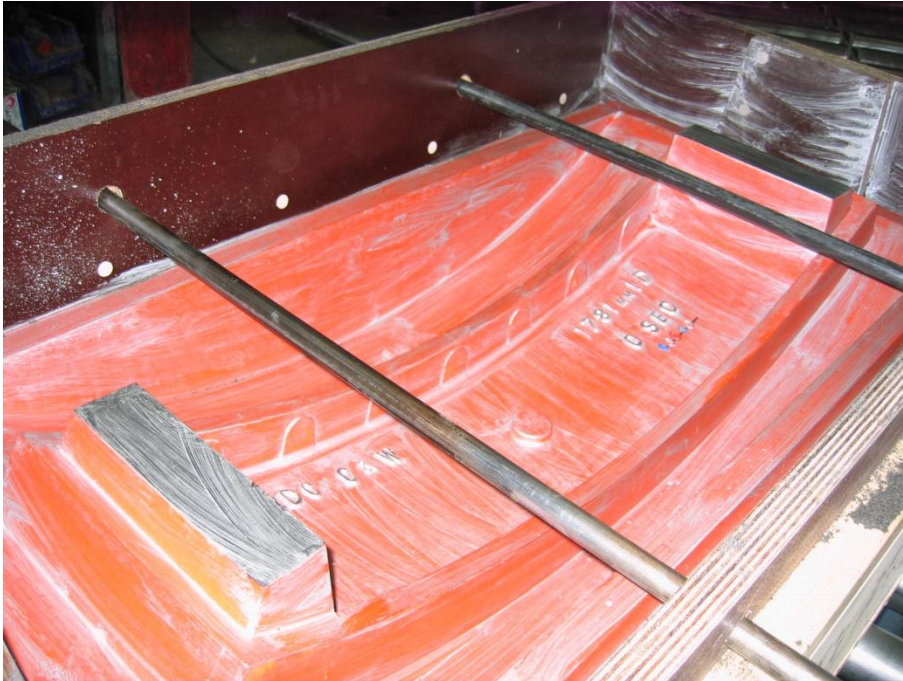
Figure 4-1. Bottom pattern for cast iron segment.
