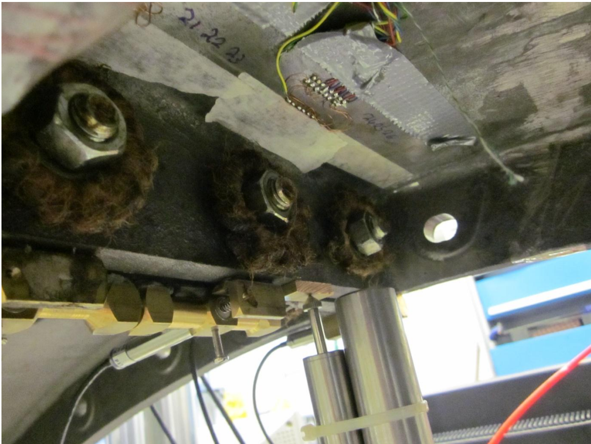
Figure 5-15. Grommets were used in the final set of tests.
