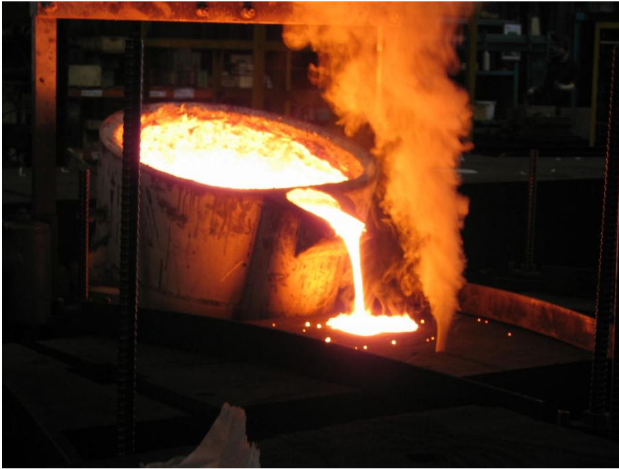
Figure 4-7. Pouring the charge mix into the sand mould.
