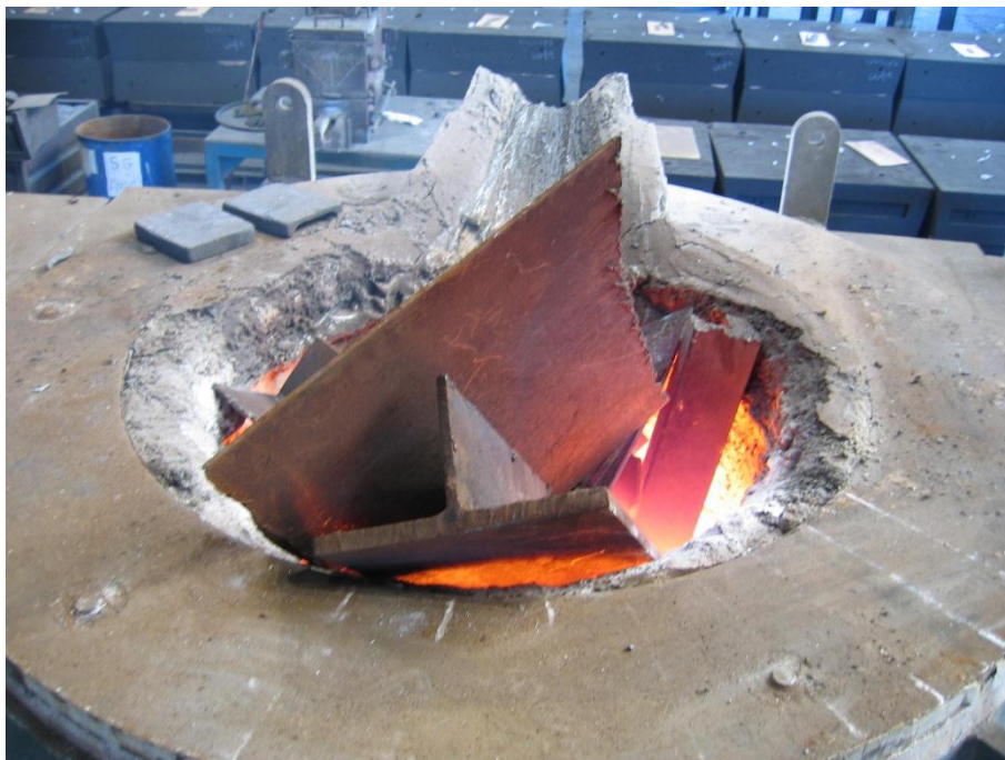
Figure 4-5. Melting the charge mix.
