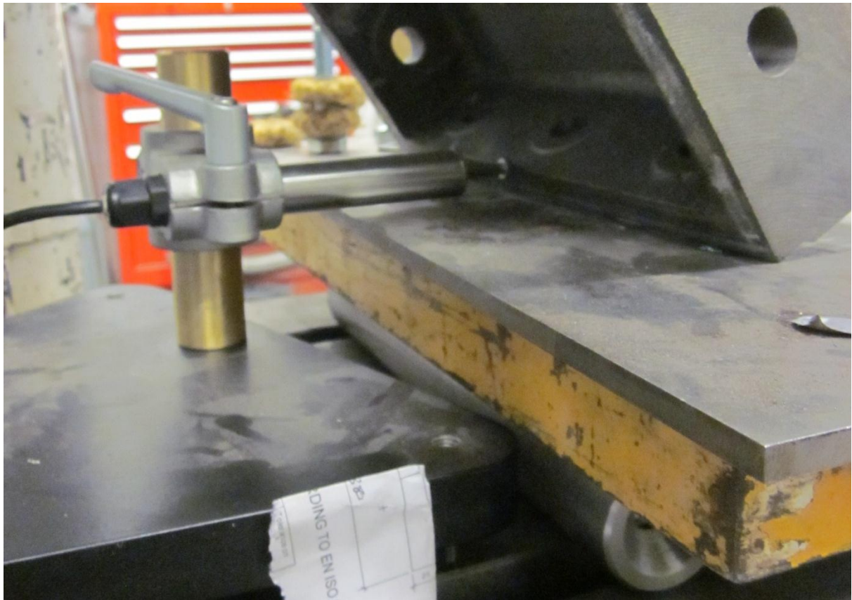
Figure 5-16. Close up view of the roller support.
