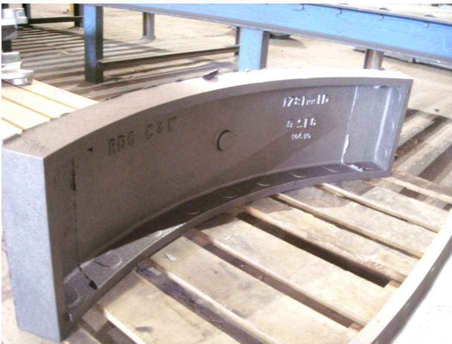
Figure 4-8. Half-scale cast iron segment prior to machining.
