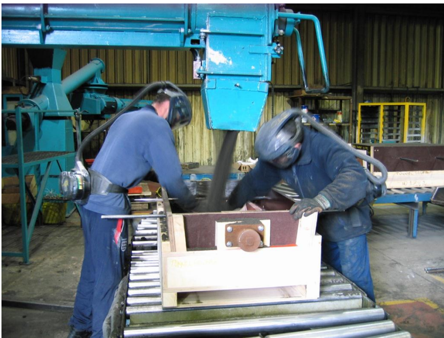
Figure 4-2. Pouring sand into bottom mould.
