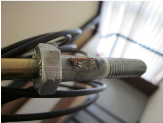
Figure 5-14. Grade 4.6 steel bolts instrumented with strain gauges.
