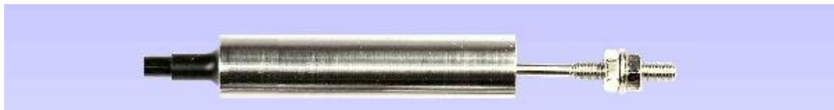
Figure 6-25. LVDT for measuring joint opening.
