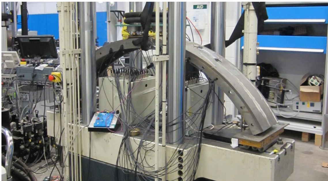
Figure 5-9. The two segment test setup at Imperial College with roller support at RHS end.
