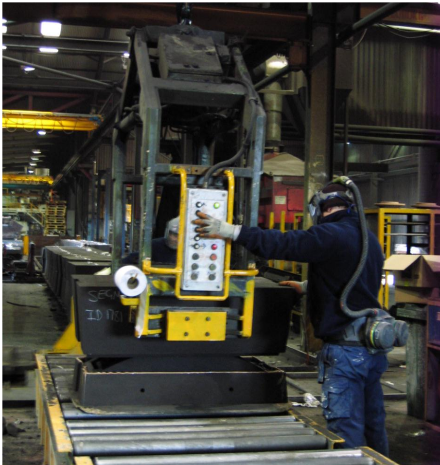
Figure 4-4. Assembling the top and bottom halves of the sand mould for a segment.
