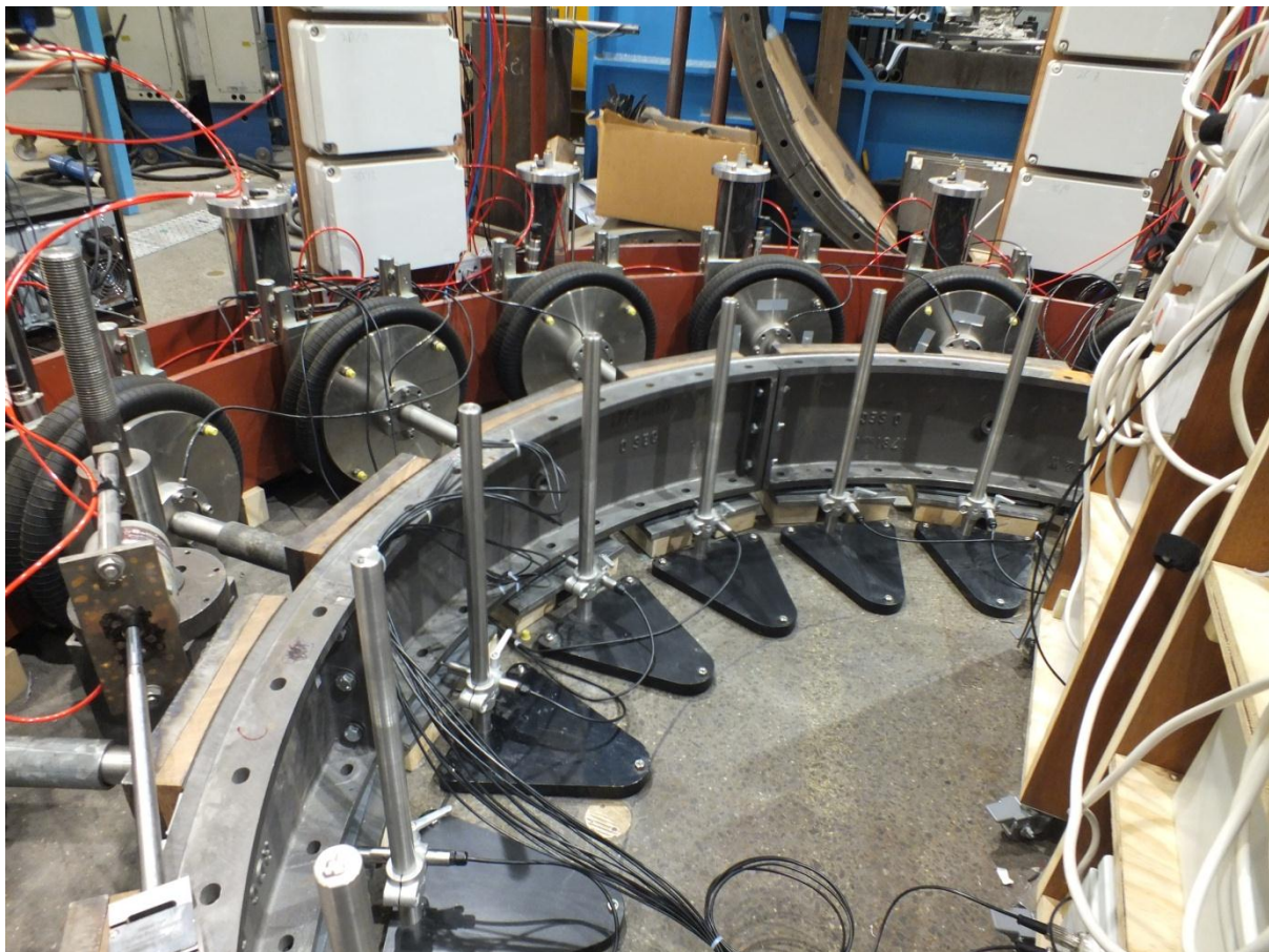
Figure 6-18. Strain gauged displacement transducers placed around the test ring.
