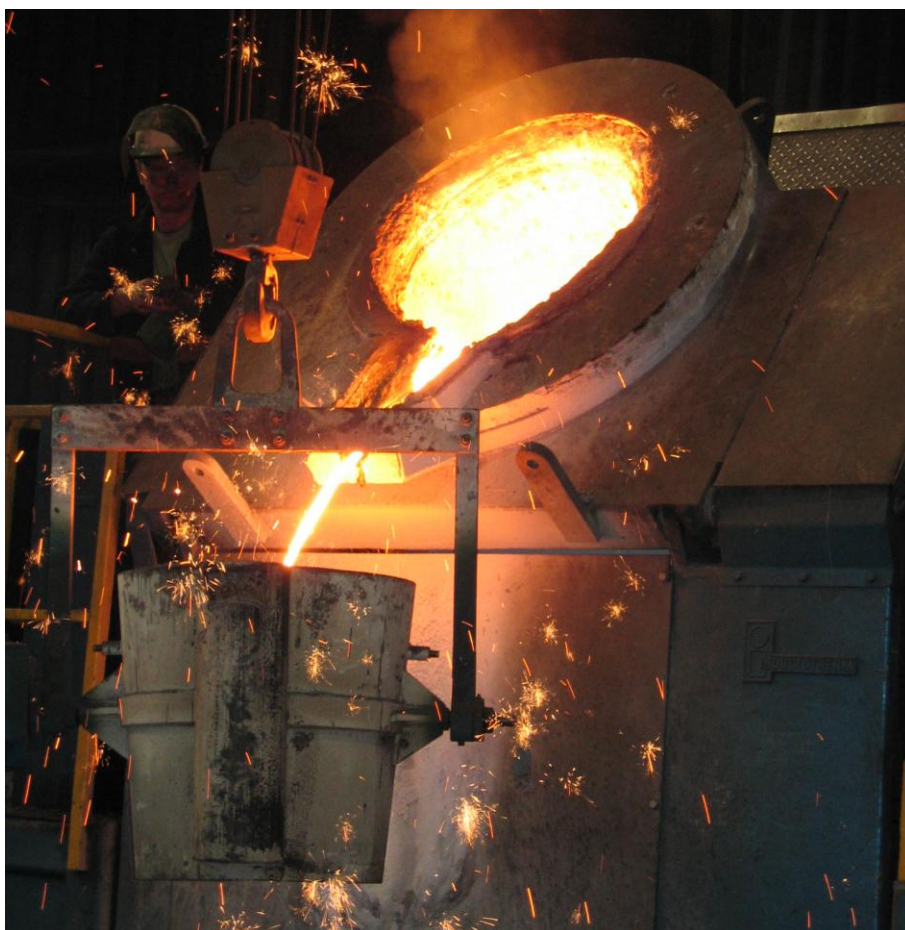
Figure 4-6. Pouring the charge mix into the ladle.
