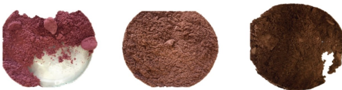
Figure 4-14. Lignins isolated with different pretreatment severity: 120 °C (left), 150 °C (centre) and 170 °C (right).
