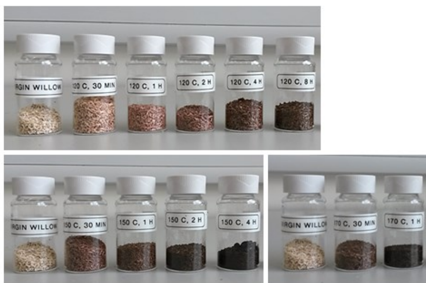
Figure 2-4. Examples of the physical appearance of raw Salix before pretreatment and pulp after pretreatment at 120 °C (top), 150 °C (bottom left) and 170 °C (bottom right) for different amount of time.
