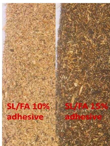
Figure 4-5. Particleboards manufactured from wood chips and a bio-based adhesive consisting of spent-liquor and furfuryl alcohol with 10% and 15% of glue. 44
