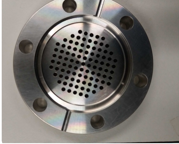
Figure 5.16: Protective DN40 flange used to shield the vacuum gauge from microwave power.
