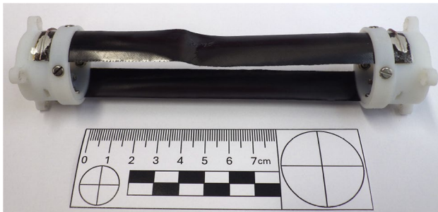
Fig. 18 Flexure 2 following the thermal failure
