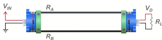
Fig. 11 Electrical schematic for power transmission test
