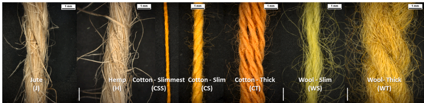
Fig. 1. Selection of natural fibre yarns; J- jute, H – hemp, CSS – cotton (super slim), CS – cotton (slim), CT – cotton (thick), WS – wool (slim), WT – wool (thick).
