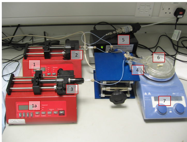
Figure 4.1: Experimental set-up for the capillary flow experiments (photograph). 1, 1a = syringe pumps; 2 = heptane in the Hamilton syringe; 3 = crude oil+toluene mixture in the Hamilton syringe; 4 = glass capillary and metal holder; 5 = pressure transducer and data acquisition system; 6 = petridish filled with water; 7 = magnetic stirrer.
