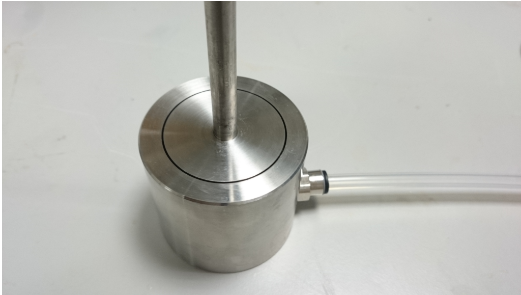
Figure 4.6: Photograph of the designed Couette mixer. The inner cylinder is attached to the stirrer and the fluids are injected and released through the plastic tubing.
