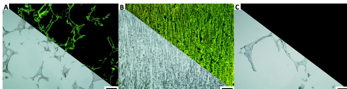
Figure 3-25. Porogen-leached (A) and directionally frozen (B) PCL scaffolds incorporating 1% (w/w) functionalized PCL-biotin and an unfunctionalised porogen-leached control for autofluorescence (C) stained with FITC-streptavidin, scale bars represent 200 \mu m.
