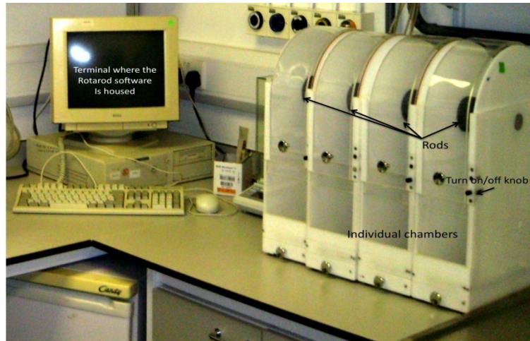
Figure 3.12: This picture shows the boxes where motion and equilibrium was assessed in mice. Up to 4 mice were assessed simultaneously and directly recorded on the local computer terminal.
