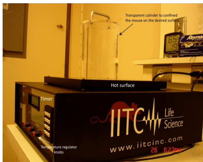
Figure 3.10: This picture illustrates the hot plate. The hot plate is used for assessment of physiological variables before fear conditioning training. The pain pathway is of vital importance as the noxious stimulus (foot-shock) is one of the components of the training paradigm used for establishing memory.
