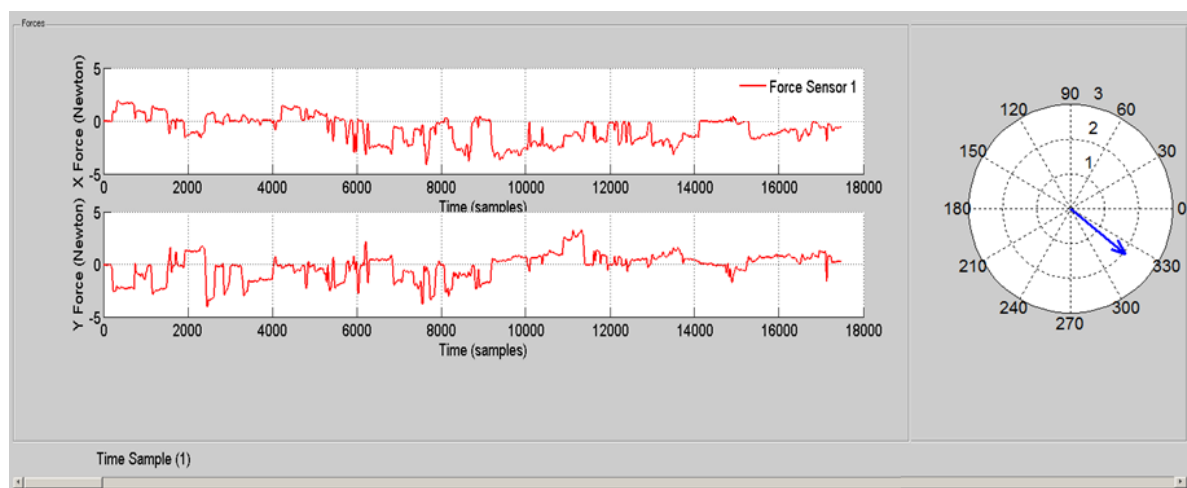
Figure 5.13; Raw data from the X and Y strain gauges for the entire length of the procedure is seen on the left. Force is highlighted in Newtons with the time in unit samples. On the right the display highlights the direction of the force for a particular time point indicated by the arrow and the magnitude by its length.
