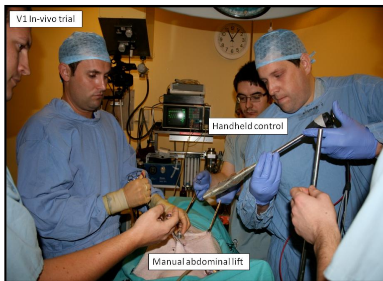
Figure 6.7; Image of the V1 in-vivo trial with the handheld prototype being steadied for insertion. A manual abdominal lift is being used to overcome the problem of sustained pneumoperitoneum.
