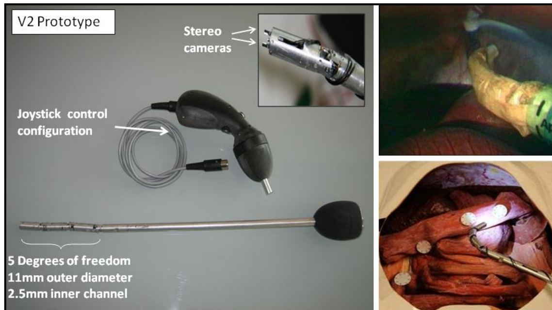
Figure 6.8; The second version prototype (V2) showing the custom made motor cables wrapped externally (inset) and its trials within the ex-vivo (bottom right) and in-vivo (top right) environments.
