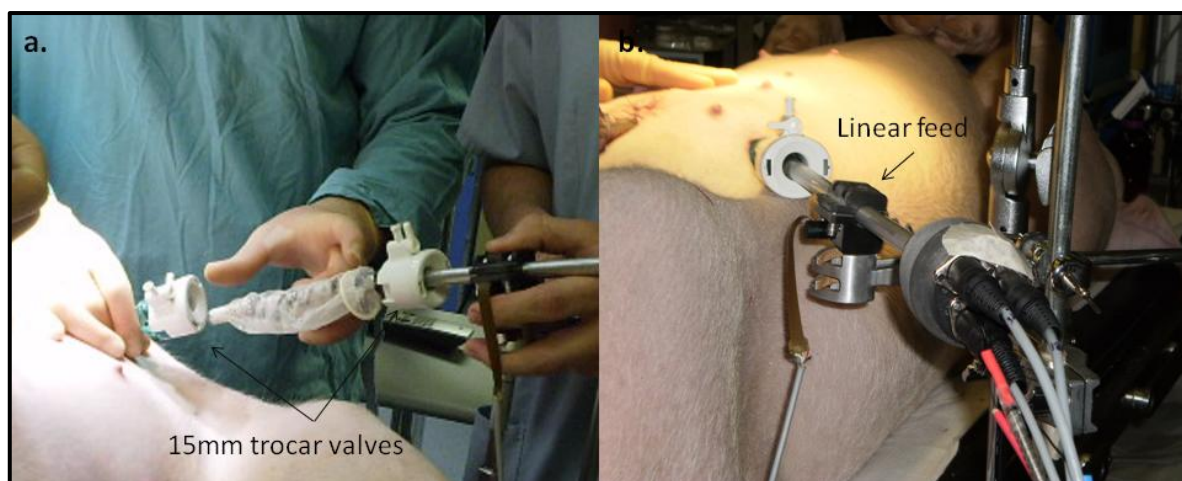
Figure 6.9; Images of the insertion and re-establishment of pneumoperitoneum with the V2. The conventional 15mm trocar valve can be seen both on the rigid section of the device and on the trocar in-situ. The linear feed mechanism can be seen in both.
