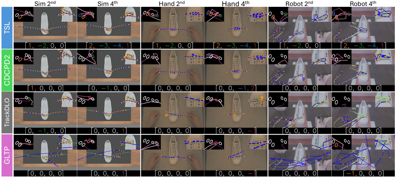
Fig. 7: Tracking results after lacing the second and fourth eyelets. Each section provides the frame image overlaid by the estimated states. Close-up views around eyelets are displayed at the top right of a section. The top left of each section presents a 3D plot of the estimated states around the eyelets, where coloured eyelets indicate that the shoelace passes through, and white indicate otherwise. The Sequential H-Signatures follow the same colour scheme as their corresponding eyelets and are shown at the bottom of each section. TSL consistently produces the correct signatures across all cases, whereas the baselines estimate the shoelace to be outside the eyelets (zero in the signatures).
