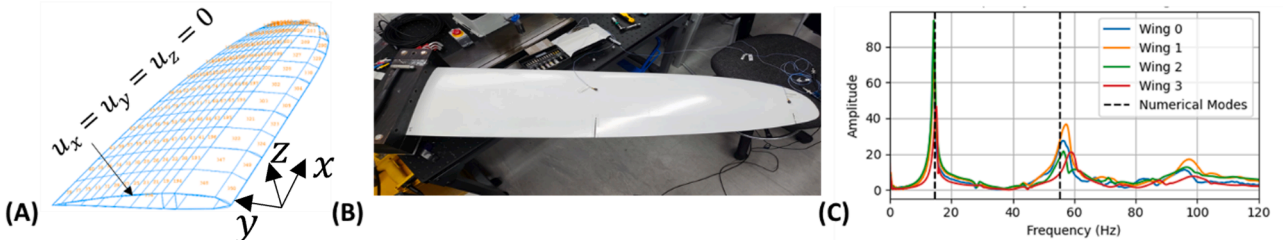
Fig. 4. A) Numerical discretization of the wing geometry using shell elements, B) experimental configuration for the extraction of acceleration time histories and C) comparison of the first 2 natural frequencies between the numerical model with the equivalent material properties and the actual wings.
