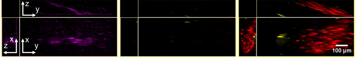
Figure 2.7 - MIPs of y-skewed volumes in live plate 1 data with erroneous trigger distance setting for the XY stage.
