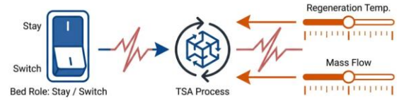
Figure 1. Illustration showing the decision variables for the TSA process in this study. The discrete binary decision v_t shown with either ‘stay’ or ‘switch’ for the bed role. The continuous decision setpoints \mathbf{u}_t are shown with ‘Regeneration Temp.’ and ‘Mass Flow’ sliders.
