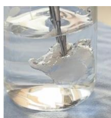
Figure 3.1.3 – A plastron layer formed around the cotton, indicating the Cassie-Baxter state [15].
