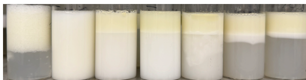
Figure 3: Visual stability assessment of a selection of rapeseed oil emulsions formulated with SDS/Span 60 blends (varying linearly from 2% to 8% SDS, left to right). The sample formulated with a 3% SDS / 97% Span 60 ratio was identified as the most stable, exhibiting minimal phase separation, thereby defining the HLB of SDS.
