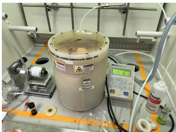
Figure 3: Spin coater used to apply the Matrimid/CPOC-301 selective layer onto PAN support membranes
