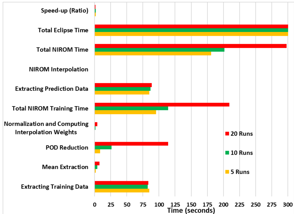
Figure 7.34: Breakdown of the average time taken to implement NIROM predictions for the seasonally varying production parameter cases of the modified Norne field with mixed production controls. Less than 0.2% of the NIROM implementation time is spent on the actual NIROM predictions/ interpolation.
