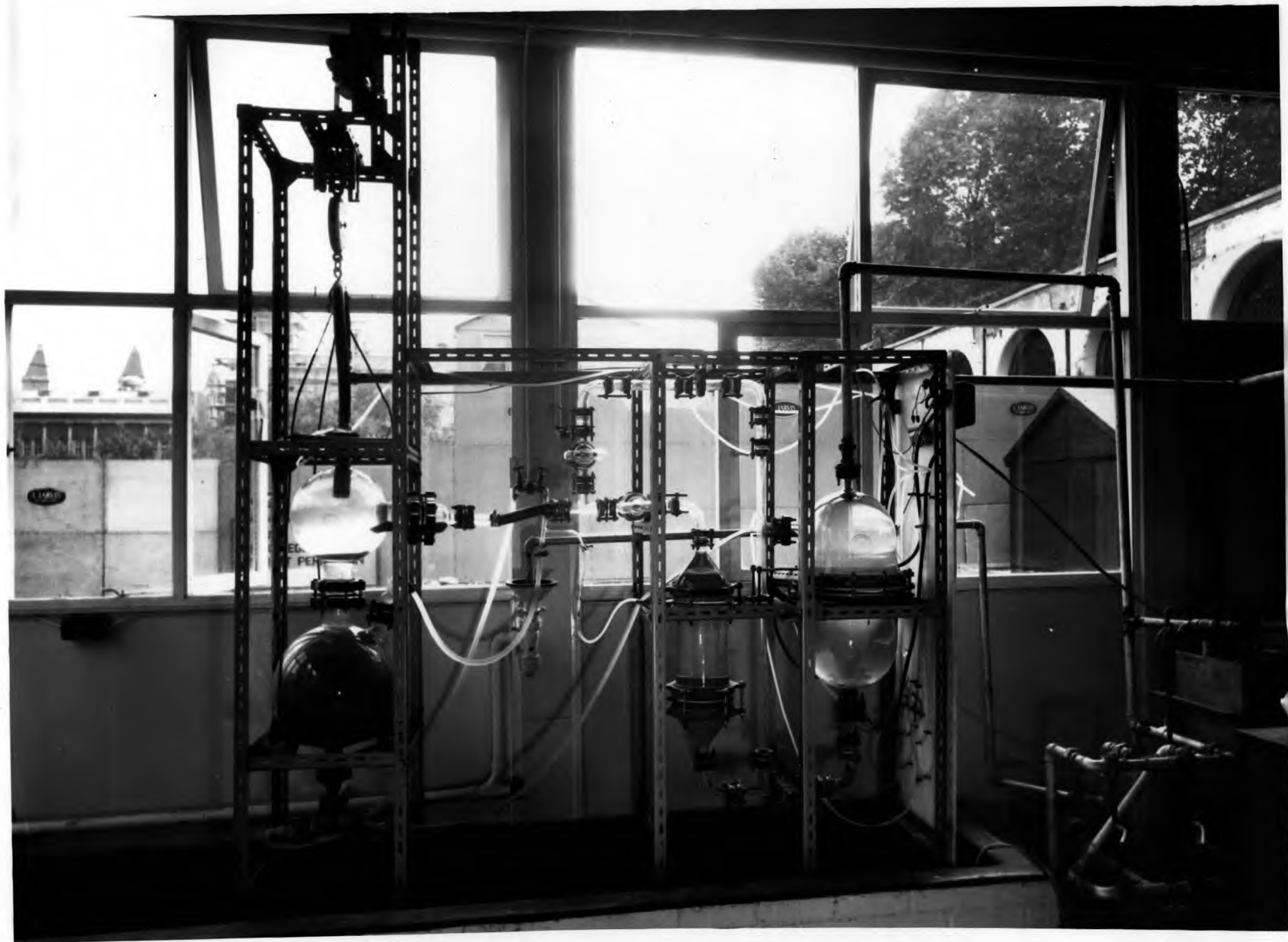
Fig. 4 Photograph of single stage contactor
