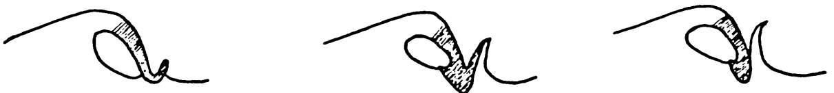
Fig. 2.23 Sketches of possible modes of splash-up after the plunging point.
