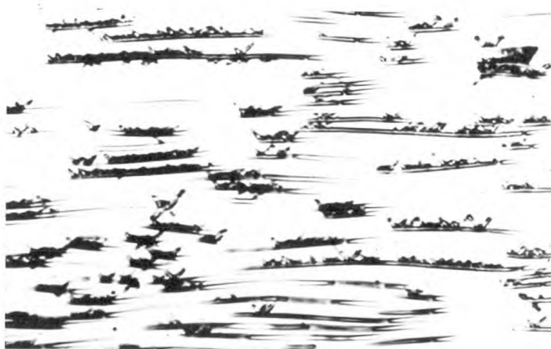
Fig. 2.36 Etch pit rows at unbroken locations along whiskers in creep tested specimen.
