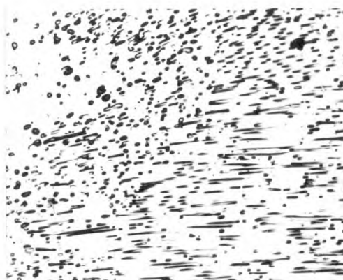
Fig. 2.33 Microstructure adjacent to composite rupture surface after creep test at 550°C.
