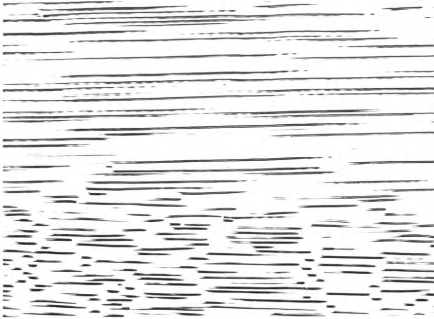
Fig. 2.6 Longitudinal section parallel to solidification axis (horizontal). R = 7.2 \text{ cm/h} (Magn. 500 X)
