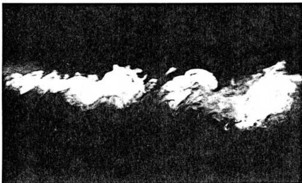
FIGURE 6. Conventional turbulence in two-stream mixing layer. Conditions as in figure 5 except that low-speed stream has been stopped completely and entrainment flow is provided by highly turbulent recirculating air. Again only a longitudinal section is illuminated.
