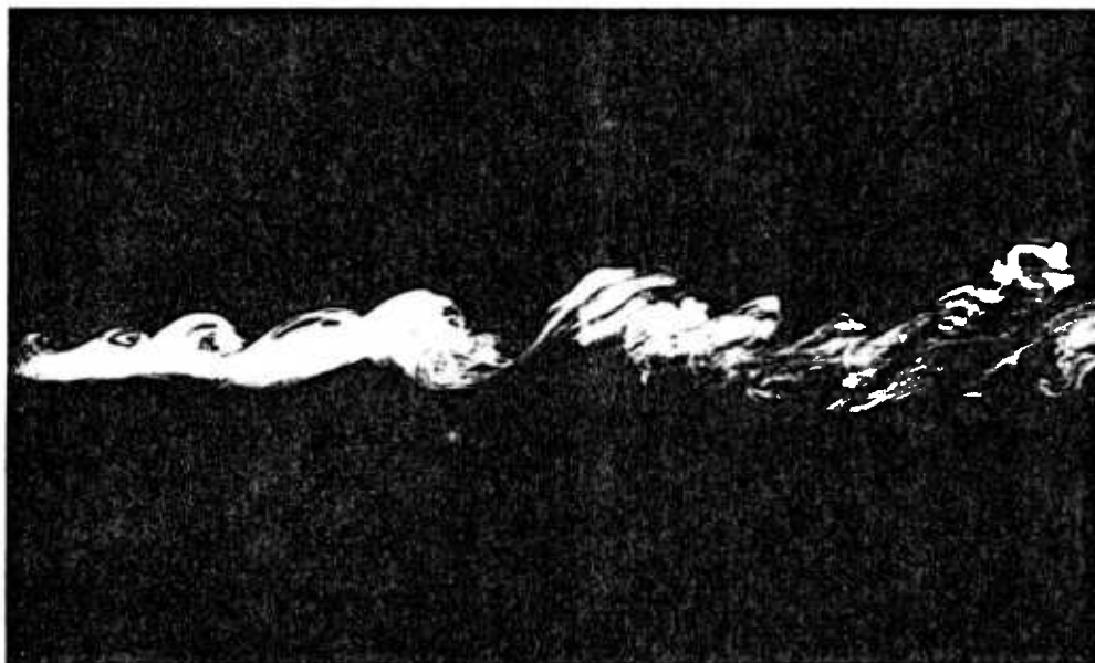
FIGURE 5. Side view of persistent two-dimensional structure in two-stream mixing layer. Stream speed ratio about 30 : 1. Reynolds number based on length of photograph approximately 60 000. Illuminated longitudinal section of smoke-filled flow.
