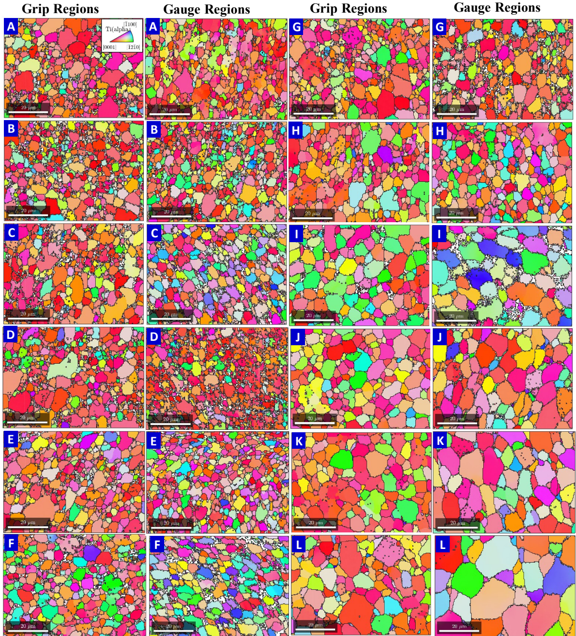
Figure 4. 7. Grain orientation maps in TA15 during static annealing and superplastic deformation. (The labels A, B, ...L denote the interrupted stages of the tensile tests)
