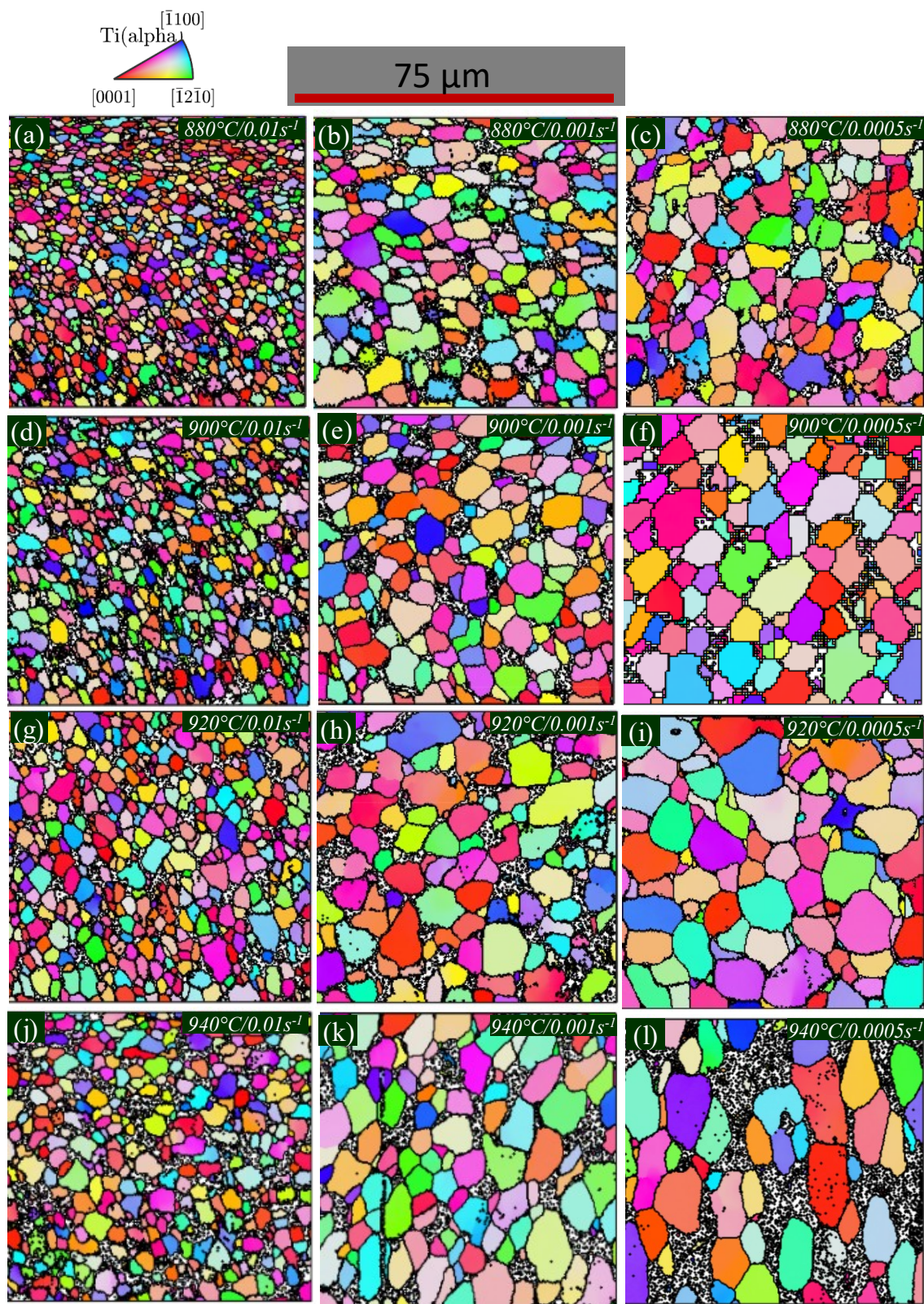
Figure 5. 7. Grain orientation maps of TA15 at final fracture points under given deformation condition
