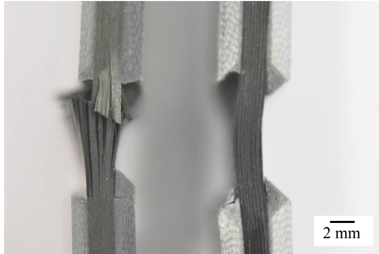
Figure 61: Failed 0° control sample (left) and interleaved composite A (right) after compression testing at 120 °C
