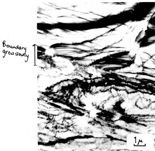
4.2.1. Alloy A. Solution treated + cooled in the electron microscope to -70^{\circ}\text{C} .
