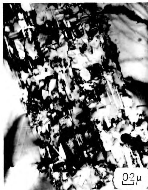
3.14.4. Alloy A. Quenched to -196^{\circ}\text{C} + 100 minutes at 560^{\circ}\text{C} .
