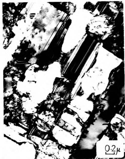
3.12.4. Alloy A. Quenched to -196^{\circ}\text{C} + 2 minutes at 600^{\circ}\text{C} .
