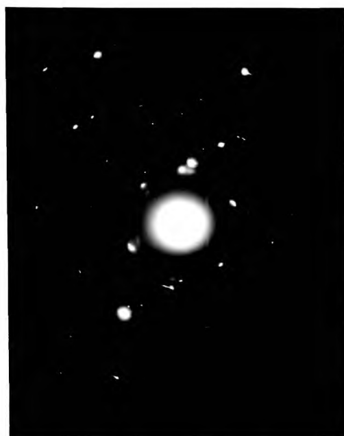
3.14.2. Alloy A. Selected area diffraction pattern taken from 3.14.1. showing a basic (110) f.c.c. pattern
