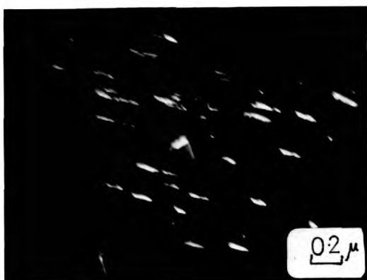
7.2.3. Alloy C. Dark field micrograph of the same region as Fig. 7.2.2. taken from a precipitate reflection
