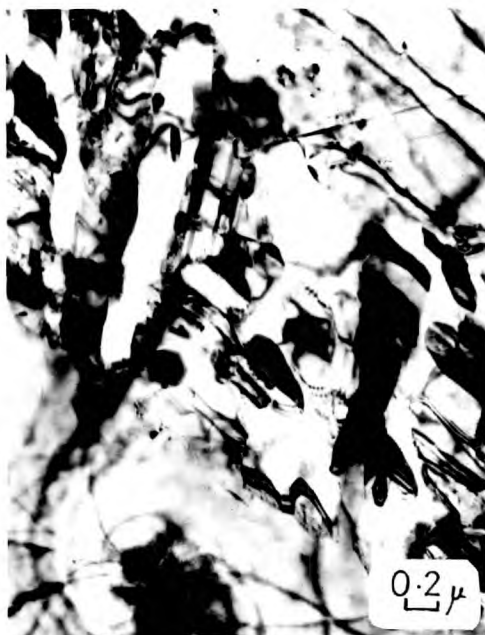
3.13.2. Alloy A. Quenched to -196^{\circ}\text{C} + 10,000 minutes at 520^{\circ}\text{C} .
