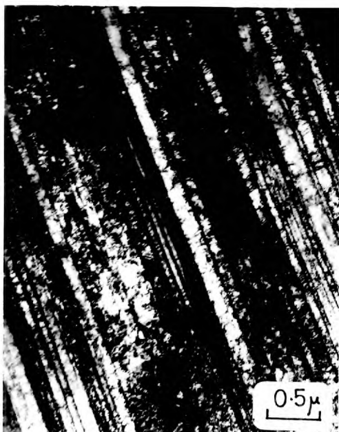
6.3.3. Alloy A. Rolled 50% at -78^{\circ}\text{C} . Transverse section.
