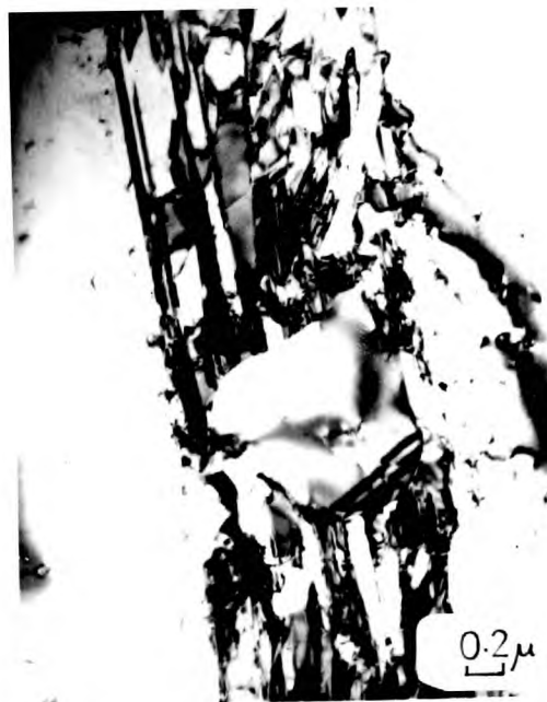
3.16.2. Alloy A. Quenched to -196^{\circ}\text{C} + 100 minutes at 560^{\circ}\text{C} .
