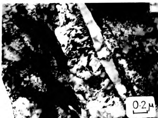
7.2.5. Alloy C. Quenched to -196^{\circ}\text{C} + 100 hours at 450^{\circ}\text{C} + 1 minute at 700^{\circ}\text{C}
