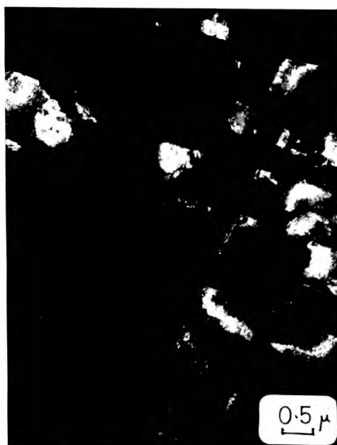
6.1.2. Alloy A. Dark field micrograph of same area as 6.1.1. taken using a martensite reflection.
