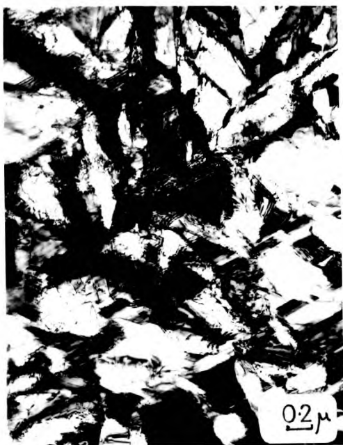
3.15.1. Alloy A. Quenched to -196^{\circ}\text{C} + 1 minute at 550^{\circ}\text{C} .
