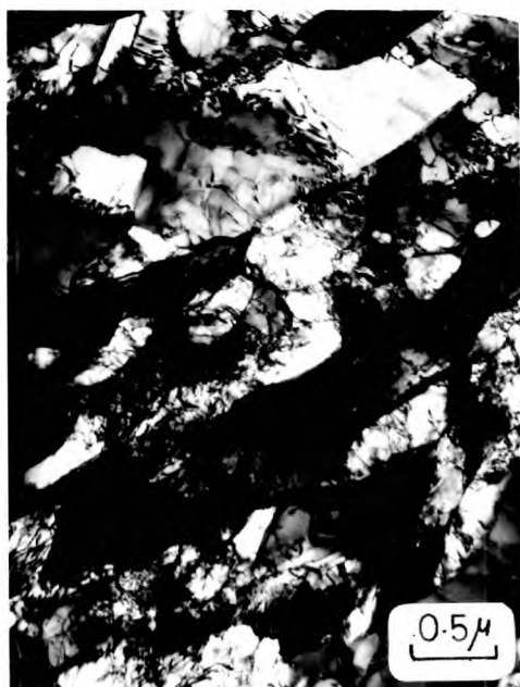
6.18.3. Alloy B. Rolled 50% at -78°C + 14 seconds at 900°C.
