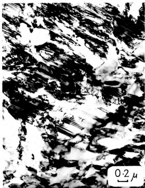
3.13.1. Alloy A. Quenched to -196^{\circ}\text{C} + 400 minutes at 520^{\circ}\text{C} .
