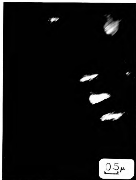
4.5.4. Alloy A. Dark field micrograph taken using a b.c.c. reflection from 4.5.2.
