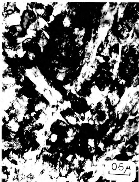
6.13.1. Alloy B. Rolled 50% at -78^{\circ}\text{C} + 2 minutes at 700^{\circ}\text{C}
