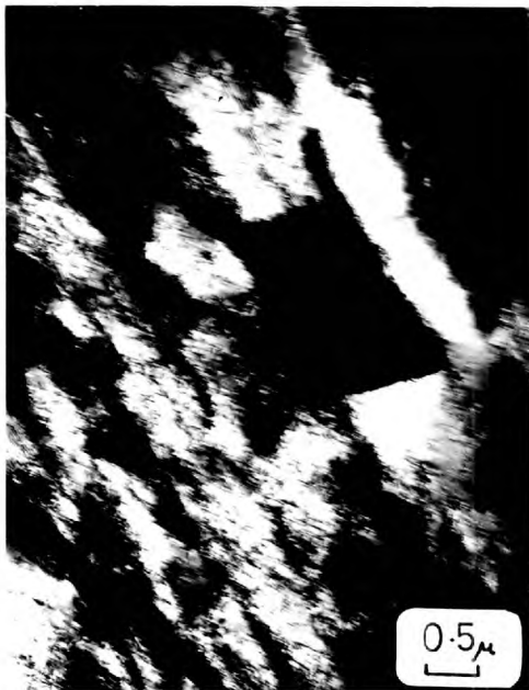
4.5.3. Alloy A. Dark field micrograph taken using an f.c.c. reflection in 4.5.2.
