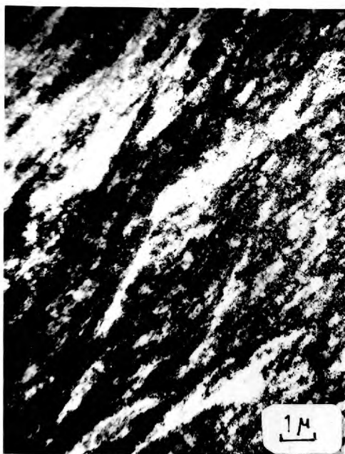
6.3.1. Alloy A. Rolled 50% at -78^{\circ}\text{C} . Longitudinal section perpendicular to the rolling plane.
