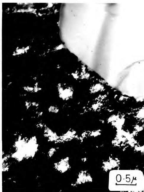
6.16.2. Alloy A. Rolled 50% at room temperature + 2 minutes at 700°C.
