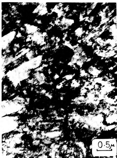
6.22.1. Alloy A. Rolled 50% at -78^{\circ}\text{C} + 2 minutes at 700^{\circ}\text{C} + re-rolled 50% at -78^{\circ}\text{C} .
