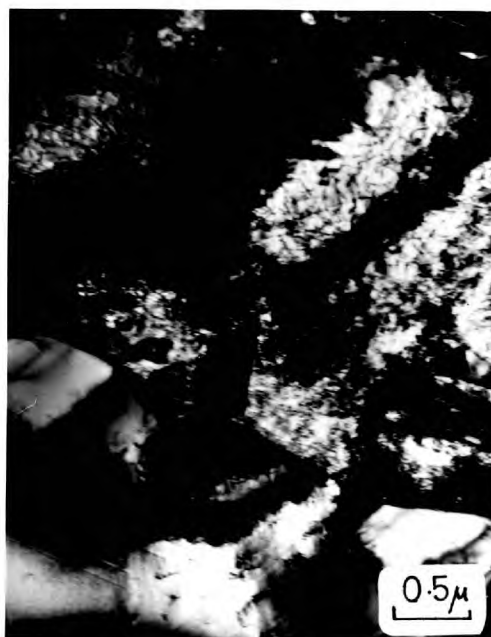
4.1.4. Alloy A. Solution treated + cooled in the electron microscope to -100^{\circ}\text{C} .
