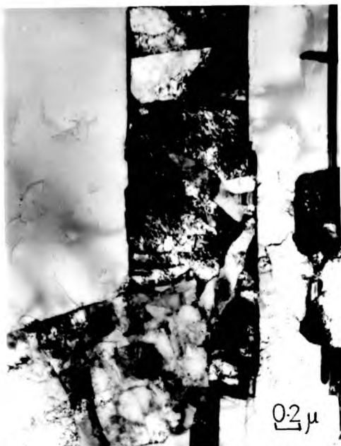
3.12.3. Alloy A. Quenched to -196^{\circ}\text{C}
