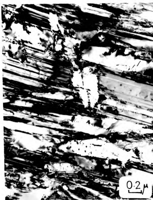
3.15.2. Alloy A. Quenched to -196^{\circ}\text{C} + 100 minutes at 520^{\circ}\text{C} .
