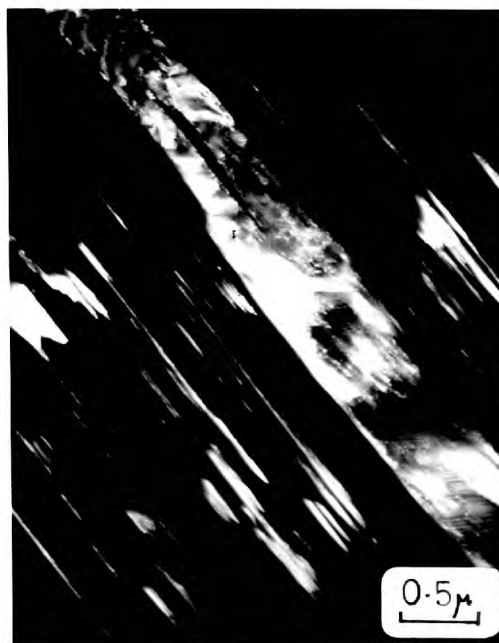
4.3.2. Alloy A. Same treatment and area as 4.3.1. Dark field micrograph taken using an austenite reflection in 4.3.3. twin related to the one used for 4.3.1.
