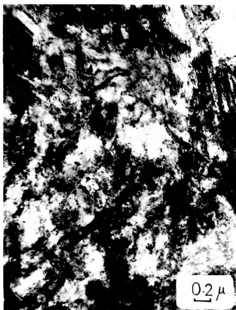
6.17.1. Alloy B. Rolled 50% at room temperature + 2 minutes at 700°C.
