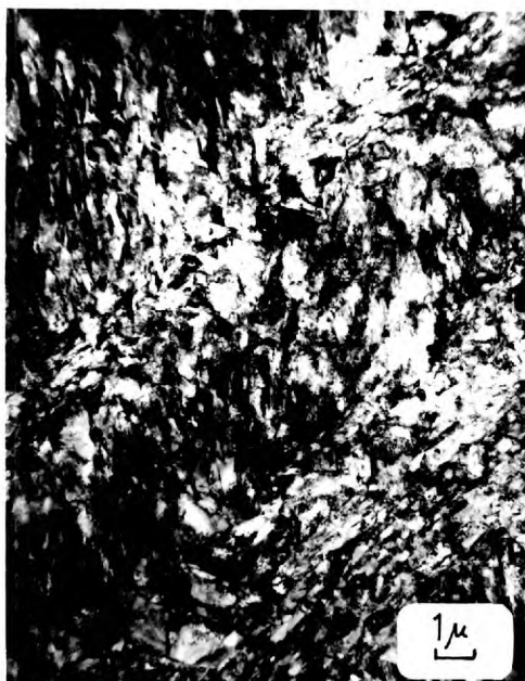
6.14.1. Alloy B. Rolled 50% at -78^{\circ}\text{C} + 2 minutes at 750^{\circ}\text{C} .
