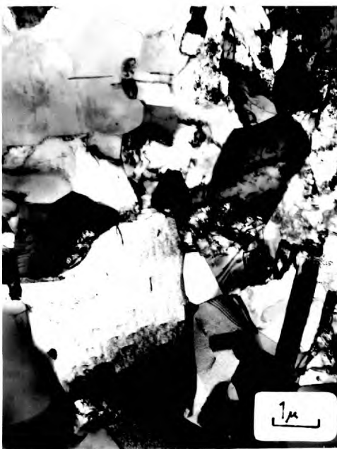
6.20.4. Alloy A. Rolled 50% at -78^{\circ}\text{C} + 20 minutes at 700^{\circ}\text{C} .
