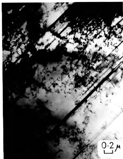
3.17.3. Alloy A. Rolled 50% at +150^{\circ}\text{C} + 1 minute at 600^{\circ}\text{C} .
