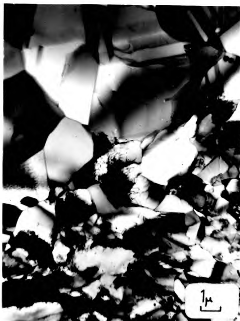
6.12.1. Alloy A. Rolled 50% at -78^{\circ}\text{C} + 2 minutes at 750^{\circ}\text{C} .
