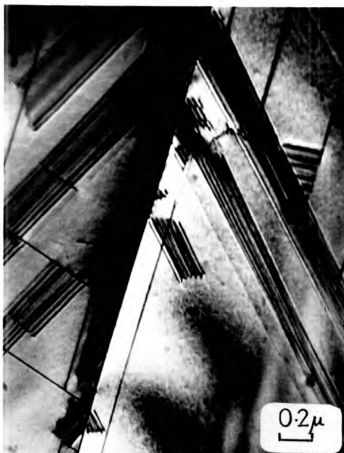
4.1.1. Alloy A. Solution treated + cooled in the electron microscope to -150^{\circ}\text{C} .
