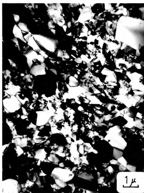
6.21.2. Alloy A. Rolled 50% at -78^{\circ}\text{C} + 7 days at 520^{\circ}\text{C} .
