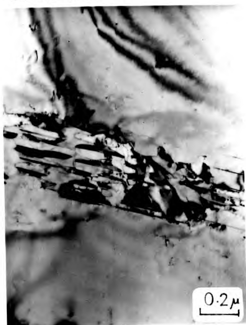
3.16.1. Alloy A. Quenched to -196^{\circ}\text{C} + 50 minutes at 550^{\circ}\text{C} .
