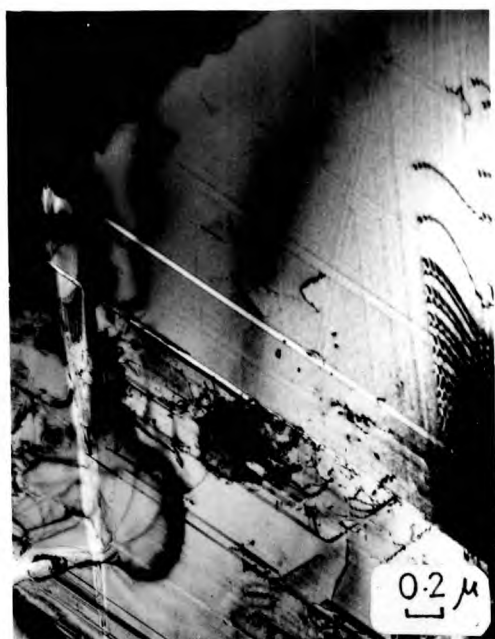
3.17.1. Alloy A. Quenched to -196^{\circ}\text{C} + 1 minute at 600^{\circ}\text{C} + 5.000 minutes at 550^{\circ}\text{C} .
