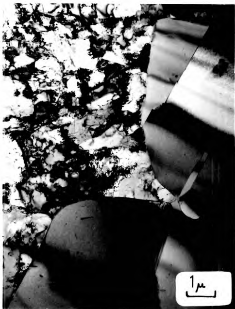
6.20.1. Alloy A. Rolled 50% at -78^{\circ}\text{C} + 10 minutes at 700^{\circ}\text{C} .
