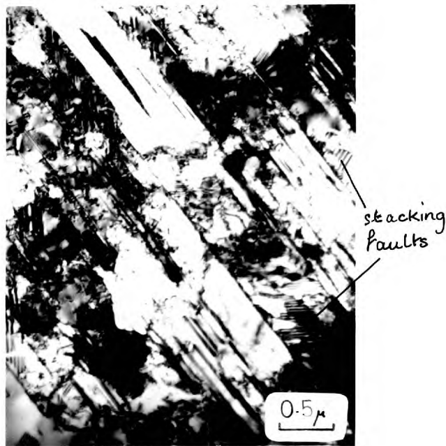
4.3.4. Alloy A. Same treatment and area as 4.3.1. and 4.3.2. Bright field micrograph.
