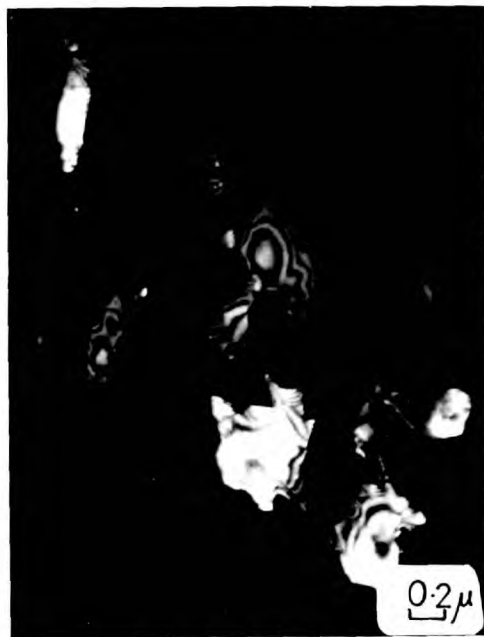
3.13.4. Alloy A. Dark field micrograph taken using a b.c.c. reflection in 3.13.3.
