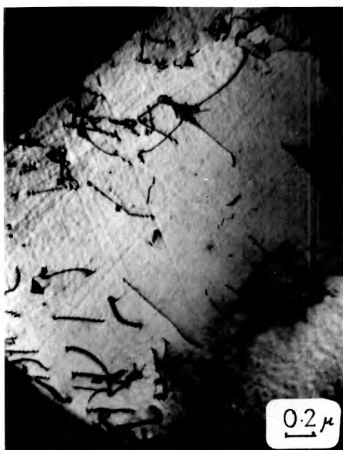
6.21.1. Alloy A. Rolled 50% at -78^{\circ}\text{C} + 35 minutes at 700^{\circ}\text{C} .
