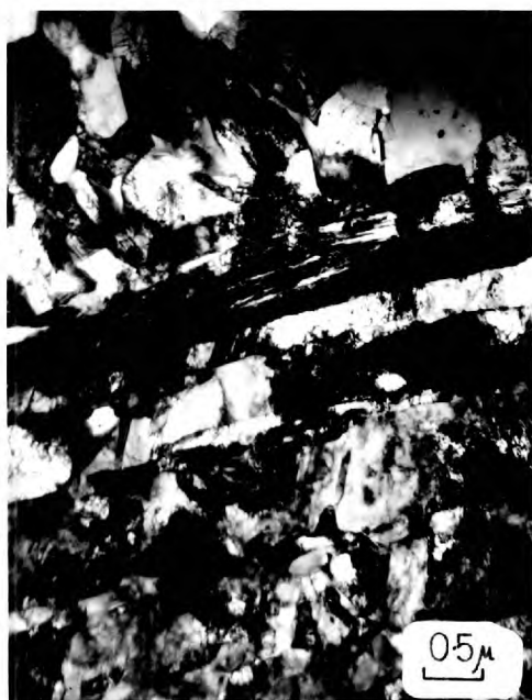
6.15.1. Alloy B. Rolled 50% at -78^{\circ}\text{C} + 2 minutes at 800^{\circ}\text{C} .
