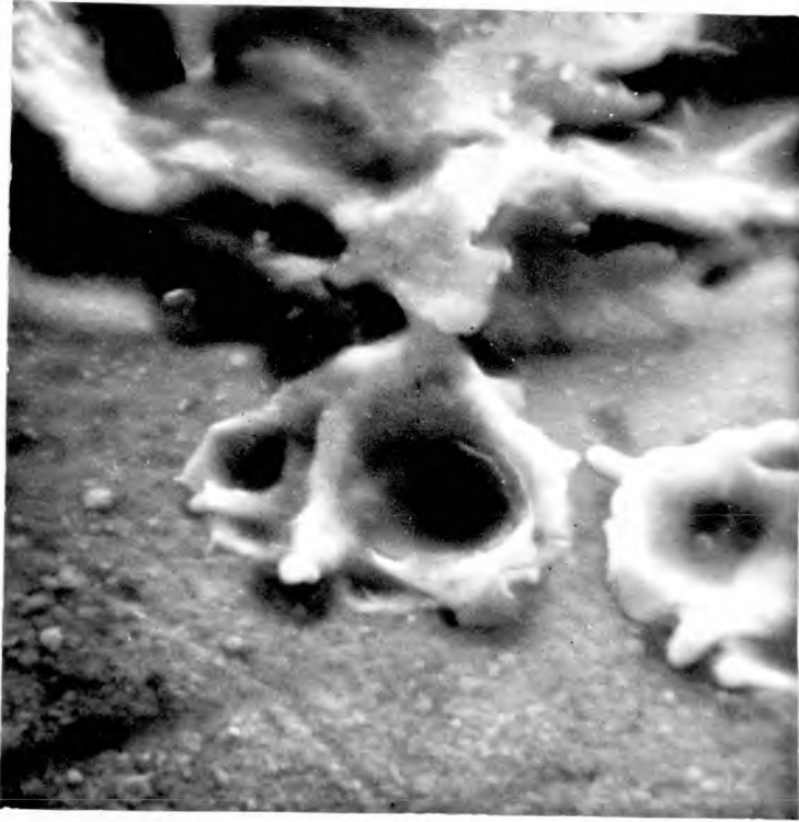
Fig. 5.10(g) Craters and overlapping of splashed material. 11,200x
