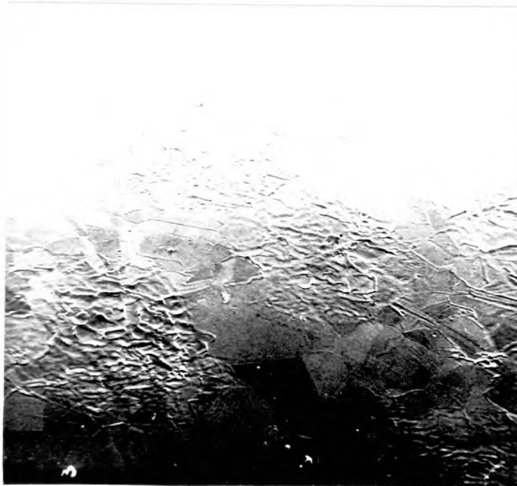
Fig. 5.9(b) Typical anode spots 70x
