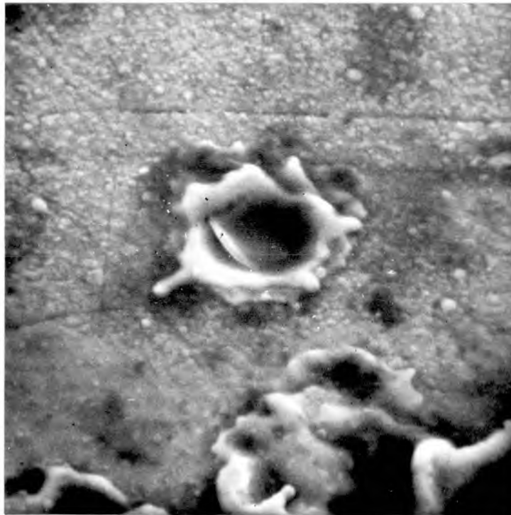
Fig. 5.10(f) Crater with splashed material 11,200x
