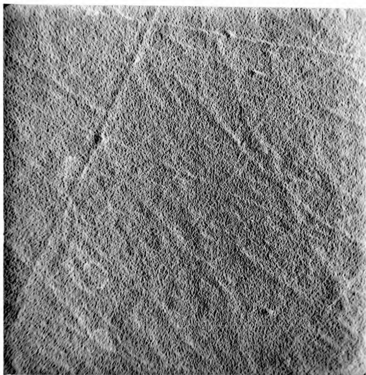
Fig. 5.9(a) Surface before breakdown tests 12000x
