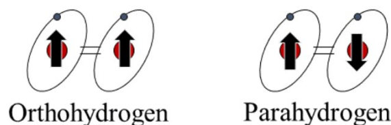
Figure 1: Diagram of the nuclear spin isomers of hydrogen
