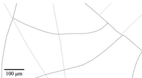
Figure 2: Processed 50x image of post-plasma plain PDMS after thresholding.
