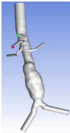
Figure 1.1 Image from ANSYS ICEM of the AAA patient specific geometry used for the project
