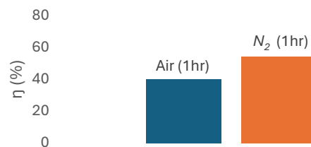
Figure 16: Photothermal efficiencies of air milled vs N 2 milled TiO 2
