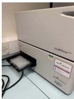
Figure 2. The set up of the CLARIOstar plate reader, where the 96-well plate is placed and inserted before beginning OD, GFP and mCrimson readings using the adjacent computer system.
