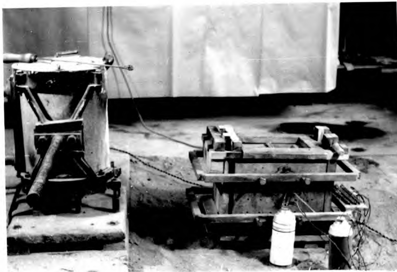
Fig. 41. Side view of Mould Assembly showing Thermocouple connections.
