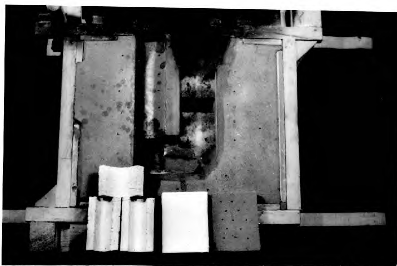
Fig. 39. View of Open Half Mould with Exothermic Cores.
