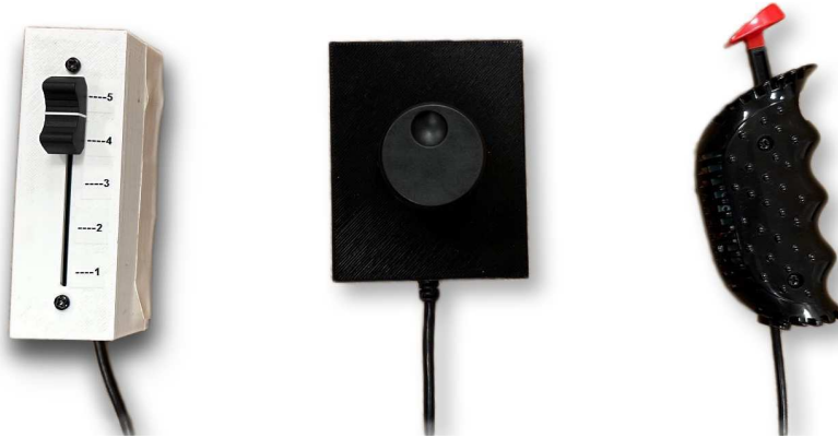
Figure 6.1: Three proposed continuous time trust measurement prototypes: a sliding scale (left), a rotary dial (center), and the final chosen device, a modified slot-car controller (right). The slot-car controller design allows participants to change their trust input intuitively and continuously, without the need for visual guidance.
