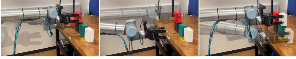
Figure 8.7: Block stacking demonstration: The UR10e robot performs a sequential manipulation task: (left) placing the red block onto the black block, (middle) retracting to reposition, and (right) approaching to grasp the white outer block for stacking onto the green block.
