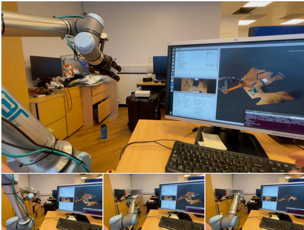
Figure 8.3: Demonstration of the ROS-based control interface combining object detection, motion planning in MoveIt, and real-time visualization in RViz. The split view shows both the physical robot and its digital planning representation (RViz) 2 .
