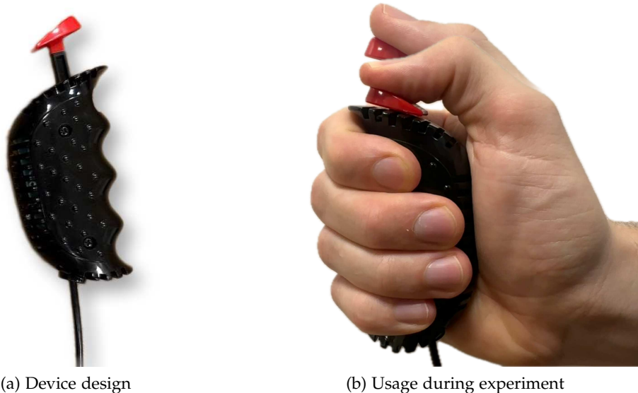
Figure 4.3: The Trusty device: (a) A modified slot-car controller repurposed for trust measurement. (b) Example usage - pressing down indicates higher trust, allowing continuous feedback during navigation without visual attention.
