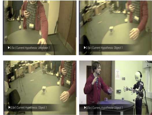
Figure 1: Experimental setup: iCub looking at target objects and arm movements (bottom right). The top-left image shows the iCub gaze following the hand. In the top-right, hand movements of the human are anticipated by the iCub gaze. Finally, the bottom-left image shows gaze focused on the target object before the hand reaches it. These three images are grabbed from the iCub camera during an interaction trial.
