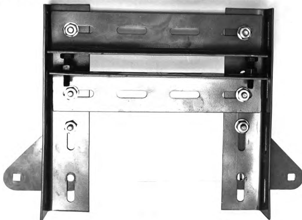
Fig. 9.2.4. Roller Support on Track for Tension Calipers.
