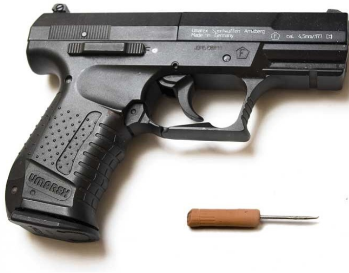
Figure 3.3 A pistol and a Z-Pin in rubber cylinder used in air gun insertion method.
