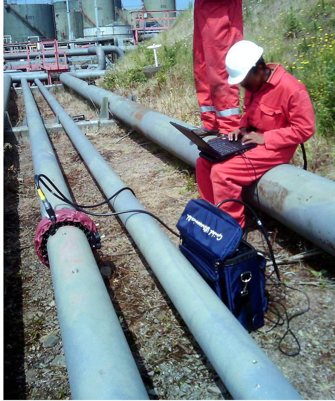
Figure 1.1.: A commercial guided wave inspection sensor produced by Guided Ultrasonics Ltd. Image courtesy of Guided Ultrasonics Ltd.
