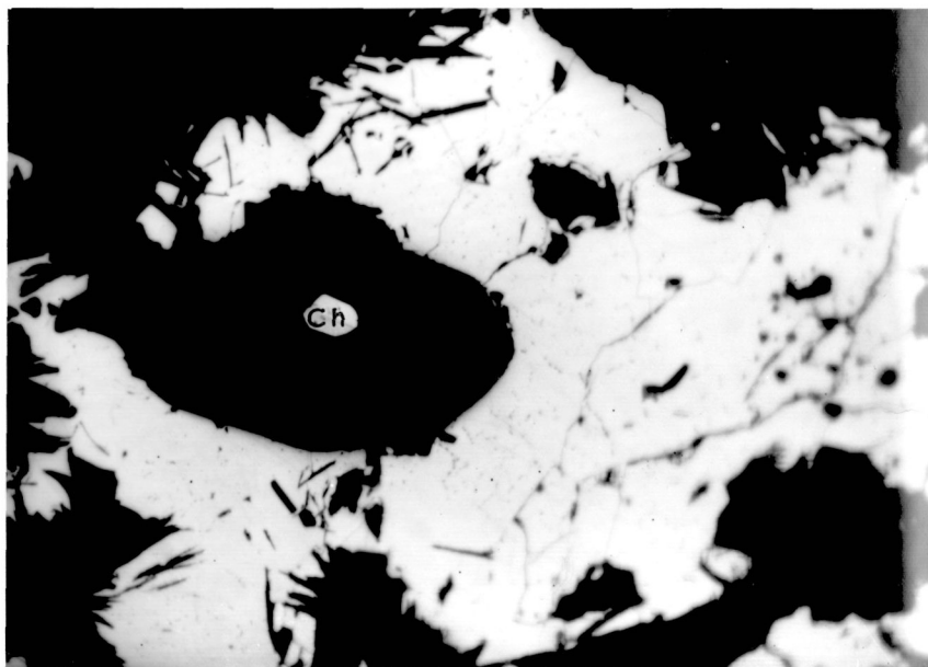
Plate 6 - (160X) Dark area of quartz (qu) surrounded by chalcopyrite (Ch) included a grain of chalcopyrite (Ch).
