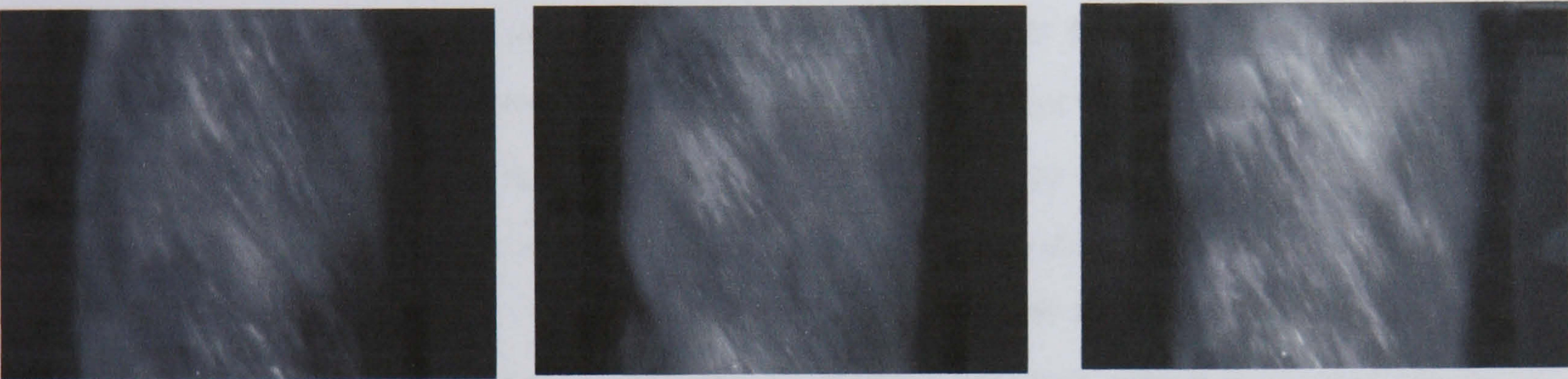
Figure 2-21 Images show the flow direction inside the transparent nozzle for 70 bar injection pressure and 1.5 ms from start of injection.
