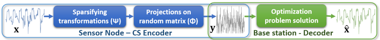
Figure 4.17: Compressive sensing information transformation flow diagram
