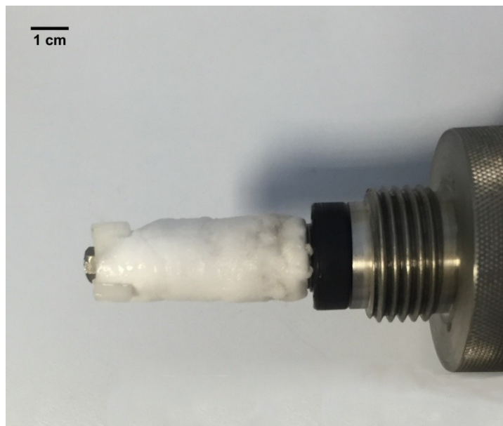
Figure 3.7 Cylindrical block of methane hydrates formed by agitating water in a methane atmosphere.
