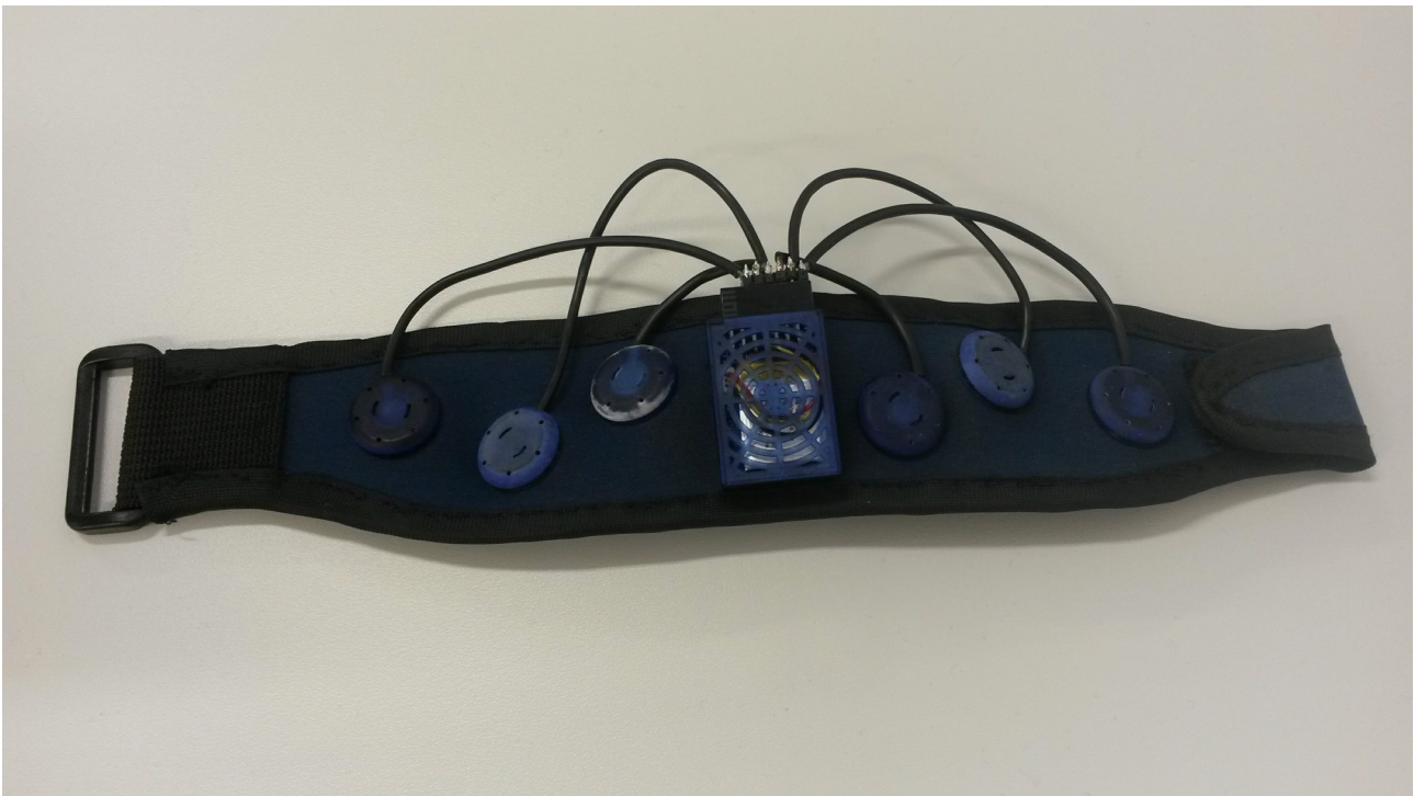
Figure 9.1: Strap used to attach an IMU and multiple MMGs to the user's forearm
