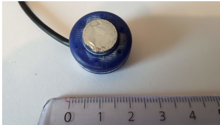
Figure 3.3: MMG external sensor used to capture muscle activity.
