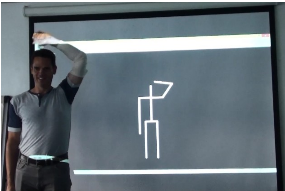
Figure 3.19: Tracking body motion using IMUs.
