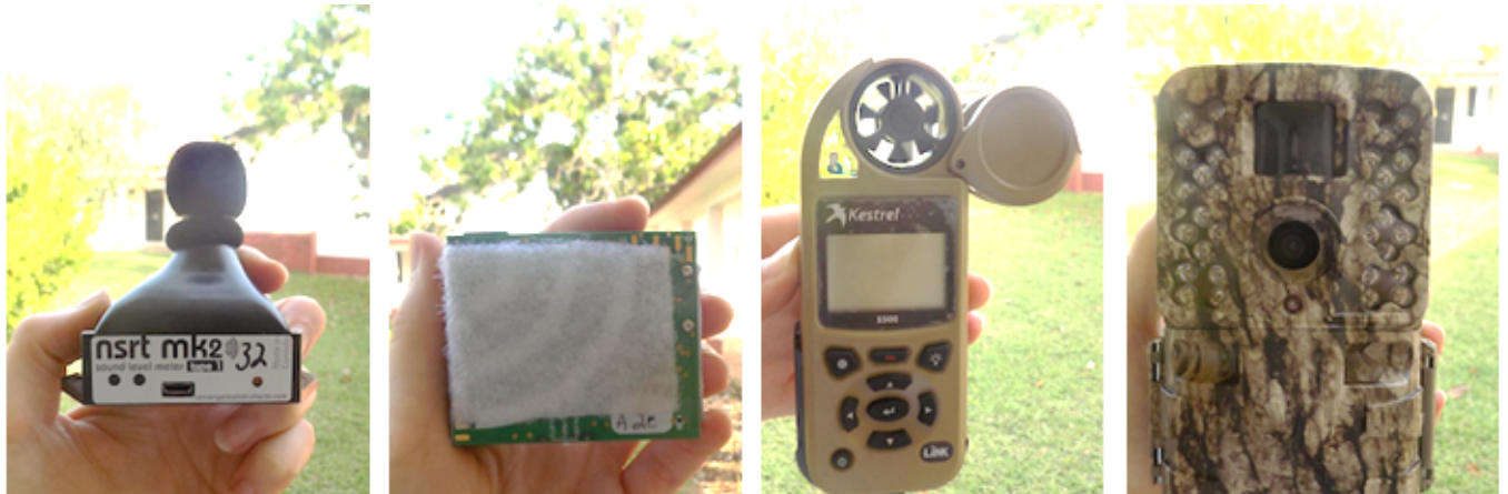
Figure 3. Sound level meter, audio recorder, weather meter, and time lapse camera. Figure is adapted from my open-access first-author paper 248 . Photo credit: Sierra Clark.
