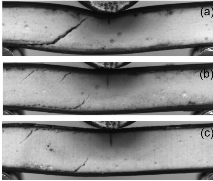
Figure 5-15 Failure modes of the (epoxy resin coated continuous UHMWPE fibre reinforced) epoxy foam core sandwich-structured composites. (a) E0 (b) E2 (c) E4
