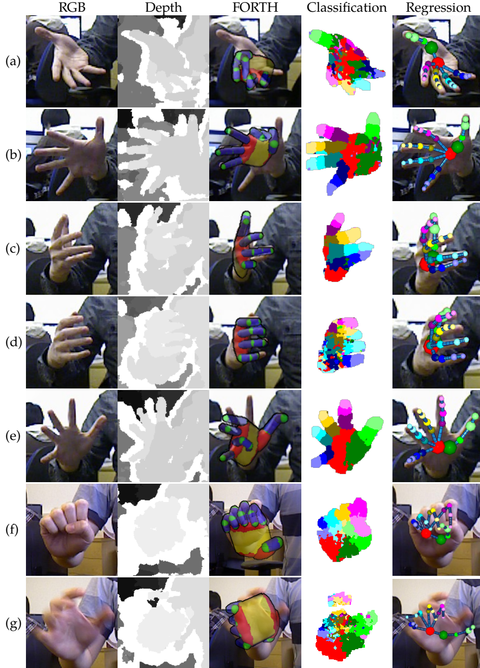
Figure 5.8: Qualitative results of the multi-view experiment. (a)-(e) are taken from sequence B and (f)-(g) are from sequence C . Hand regions are cropped from the original images for better visualisation ( 135 \times 135 pixels for sequence B , 165 \times 165 pixels for sequence C ); the size of the origin images (RGB and depth) is 640 \times 480 pixels. Colour scheme of joint labels refer to Fig. 5.4.
