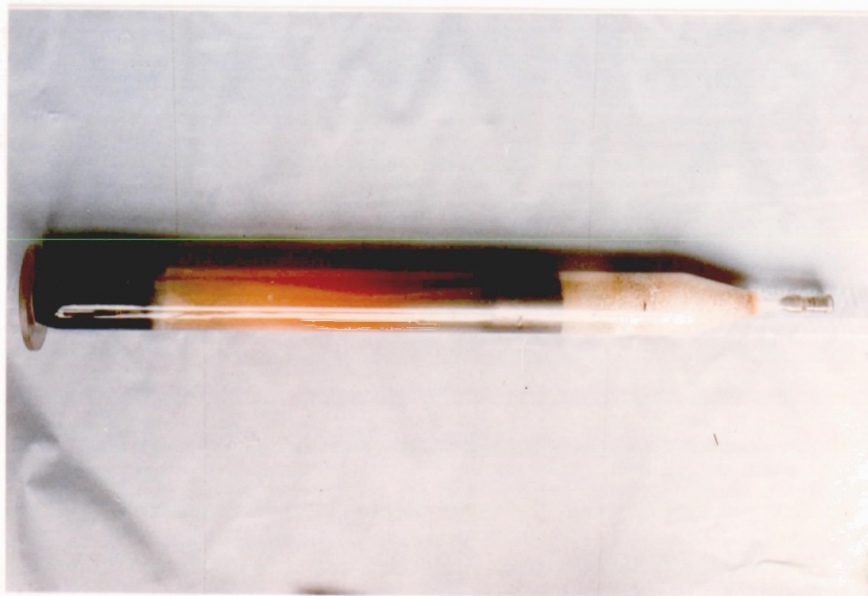
(b) Deposits On The Spouted Bed Walls After Coal Combustion
