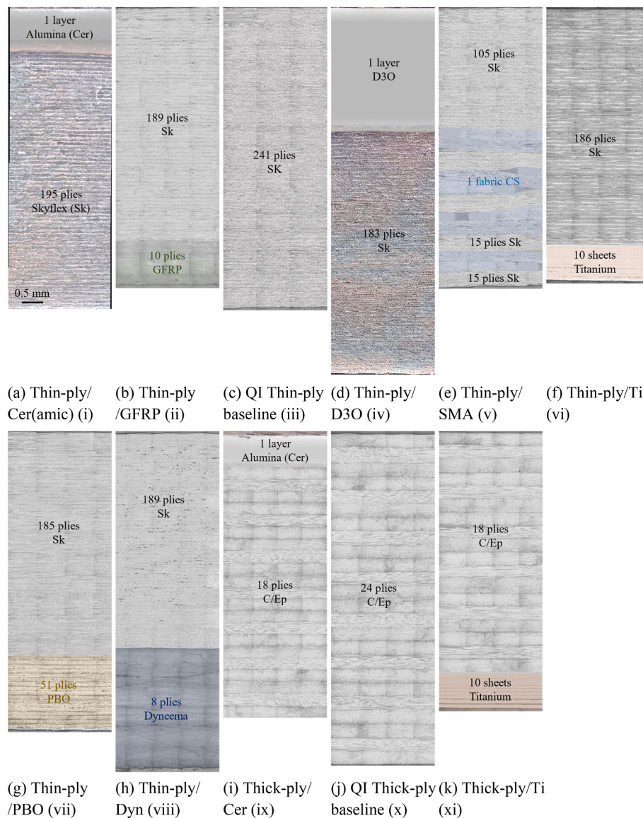
Fig. 2. Cross-sections of manufactured thin- and thick-ply laminate concepts (scaled).
