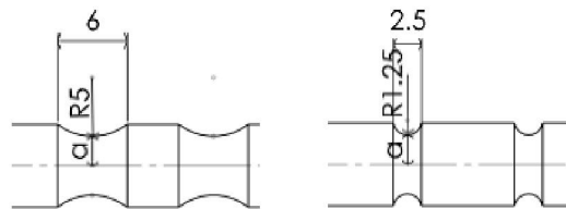
(c) Double notched (DN) sample dimensions for samples DN_R5 (left) and DN_R1.25 (right)
