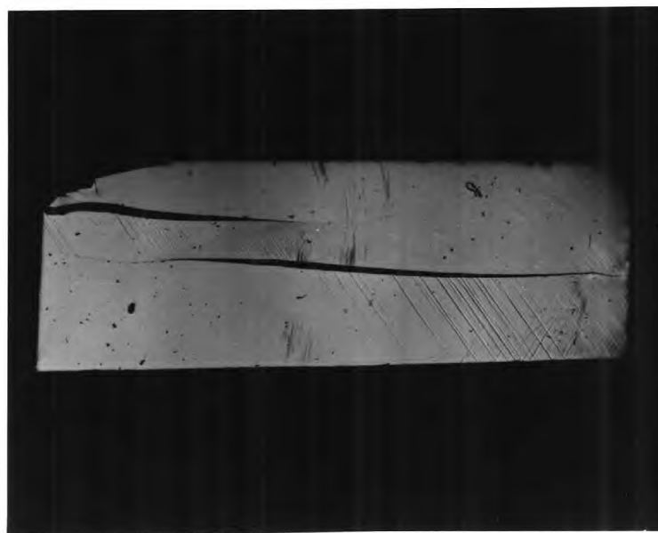
Fig. 3.8 Coarse Slip Traces at 77°K (x 11).
