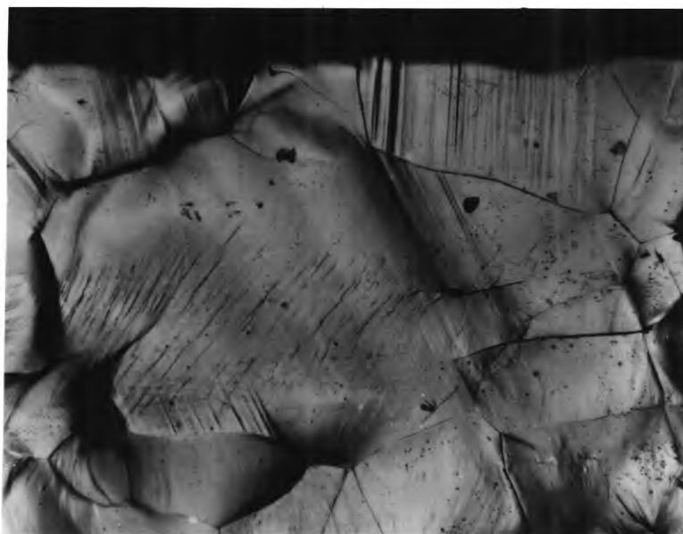
Fig. 3.20 Slip Markings in an Aluminium-Rich Polycrystal Deformed at 850°K (54 at.% Al) (x 75).
