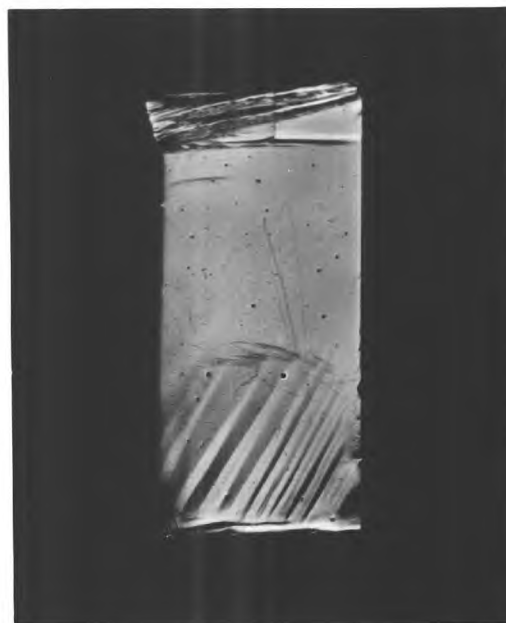
Fig. 3.33 Kinking and Transformation in a Hard Crystal at 420°K (x 11).
