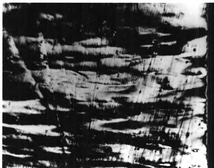
Fig. 3.13 Coarse Slip Markings on a "Screw" Face after Deformation at 195°K (x 75).
