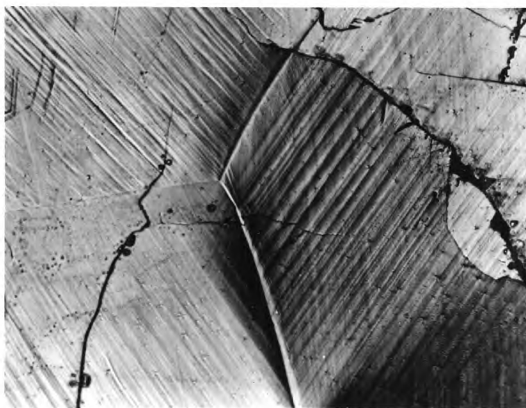
Fig. 3.17 Wavy Slip Traces on a "Screw" Face after Deformation at 550^{\circ}\text{K} (x 380).
