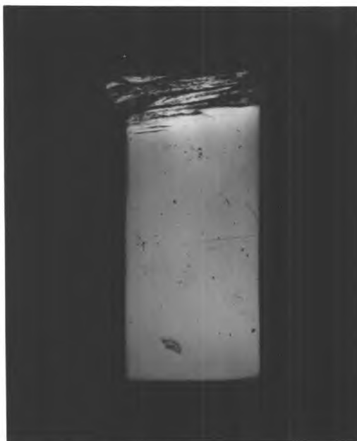
Fig. 3.32 Kinking of a Hard Orientation at 376°K (x 11).
