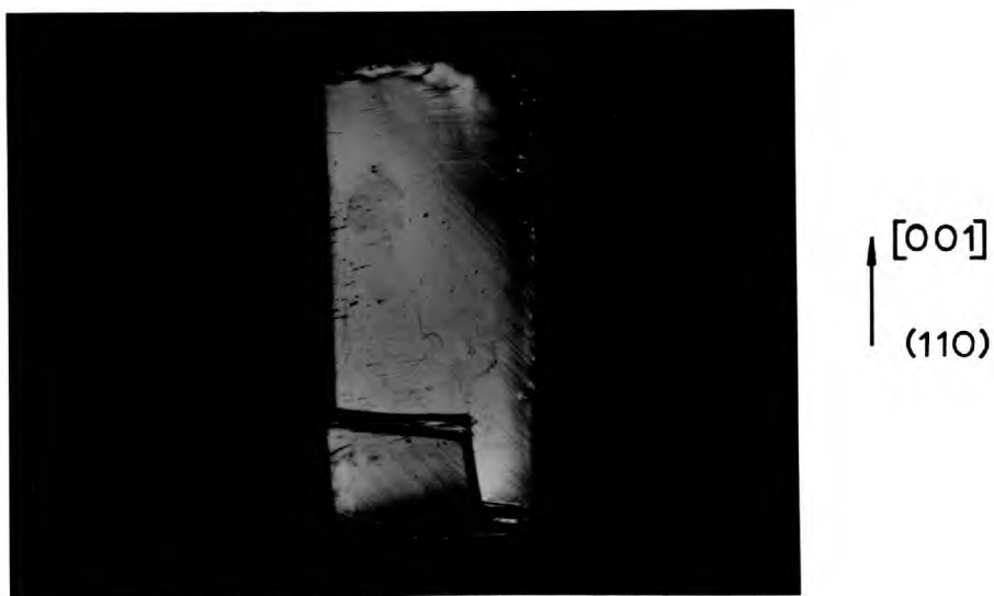
Fig. 3.41 Crack Formed at a Kink in a Hard Crystal (x 11).
