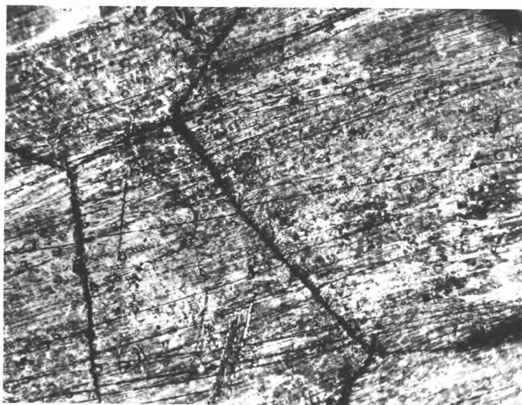
Fig. 3.25 Grain Boundary Sliding in Ni 54 at.% Al Deformed at 1075°K (x 840).
