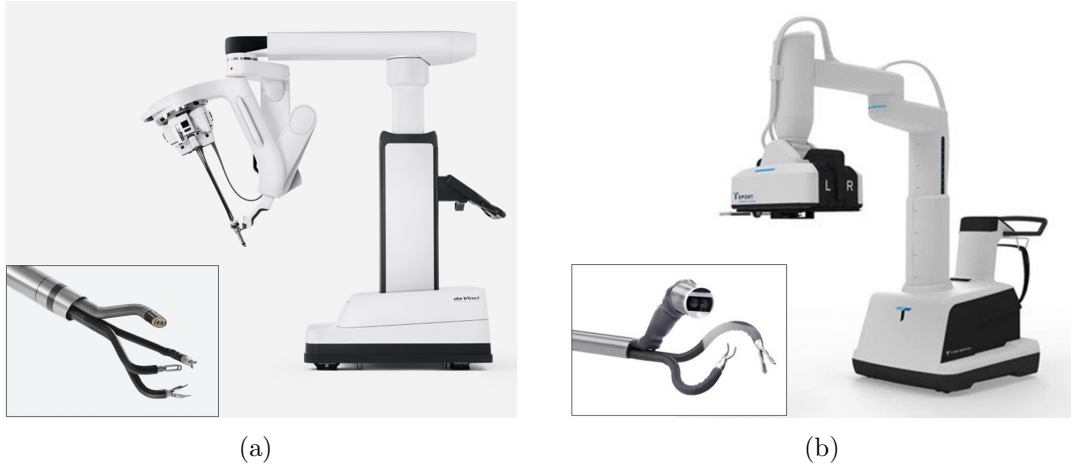
Figure 2.3: Two of the representative single-port robotic platforms, both of them share similar configurations of vision unit and manipulation arms. (a) The da Vinci SP surgical system (image courtesy of Intuitive Surgical). (b) SPORT (image courtesy of Titan Medical Inc.).
