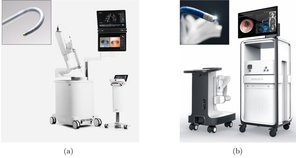
Figure 2.7: The robotic-assisted platforms for bronchoscopy. (a) The Ion endoluminal system (image courtesy of Intuitive Surgical). (b) The Monarch platform (image courtesy of Johnson & Johnson MedTech).
