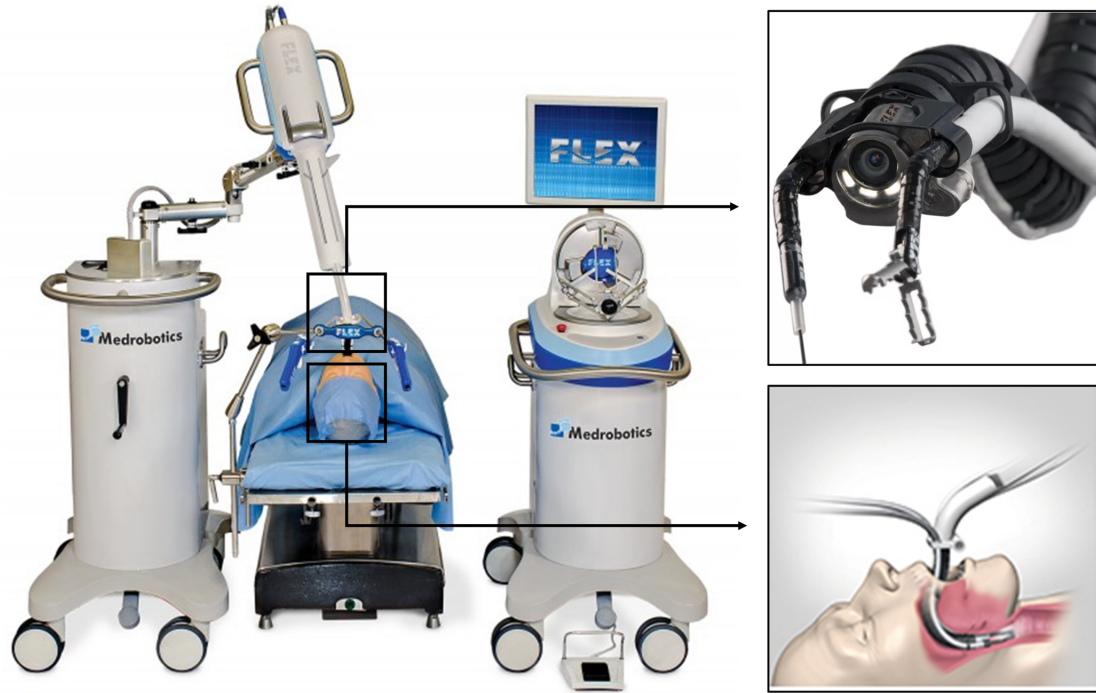
Figure 2.6: The Flex ® robotic system consists of two main units: The patient's cart and the console. The details of the robot can be viewed that the body is connected by a series of spherical joints and with function channels on the side (top right). The robot can demonstrate the follow-the-leader manner (bottom right). (Image courtesy of Medrobotics).
