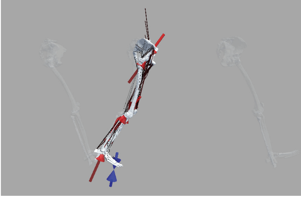
Figure 2.5: Freebody visualisation of toe-off with muscle lines of action, joint contact and ground reaction forces
