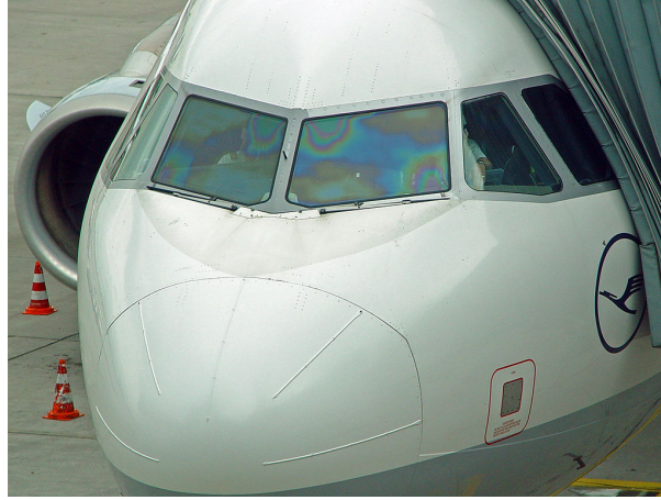
Figure 6.2: Thin-film interference pattern observable on cockpit window due to thin layer of ITO used for electrical heating. ("LHcockpitWindow" by Etan J. Tal is licensed under CC BY-SA 3.0)
