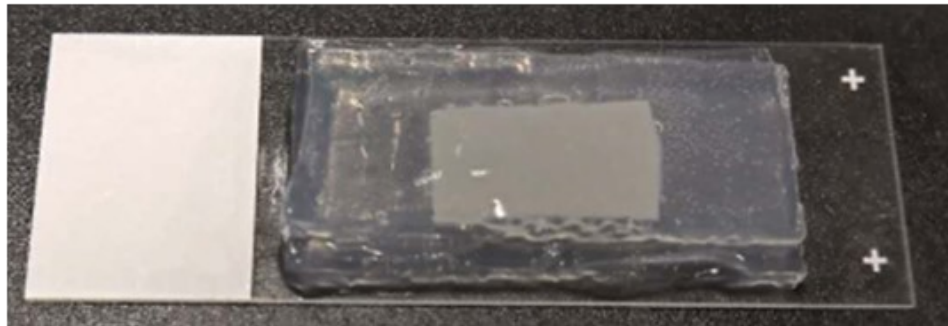
Figure 2-4 Setup to visualise light distribution from the optical fibre with a stack of gels. A thin sheet (800 \mu\text{m} ) of brain phantom gel containing 1% agarose in PBS (w/v), 0.3 \text{mg ml}^{-1} FITC-dextran (M.W.: 4 kDa), 8% dried skimmed milk powder and 0.1% liquid Indian ink (v/v) was sandwiched by two 0.5% (w/v) agarose PBS gel blocks, placed on a glass microscopy slide. A: top view of the gel stack. B: Side view of the gel stack.
