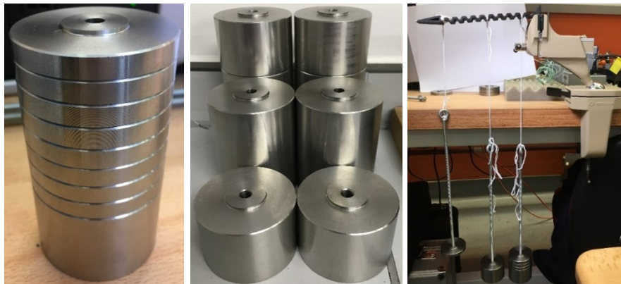
Figure 5.53. Mild steel cylinders which were in-house manufactured and were used in the static test of the CF composite corrugated structure.
