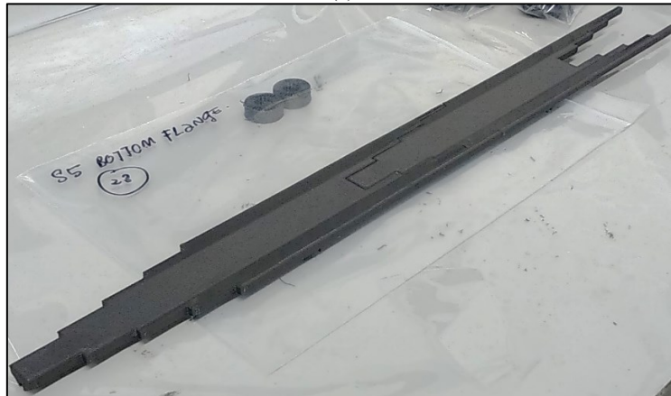
Figure 6.19. 3D-printed bottom flanges of section S5 with the scarf joint, having steps across the flange width: (a) two printed parts and (b) the combined two parts through the scarf joint.
