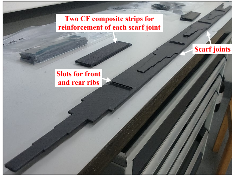
Figure 6.23. Four of the 3D-printed CF composite spar webs after several design iterations.
