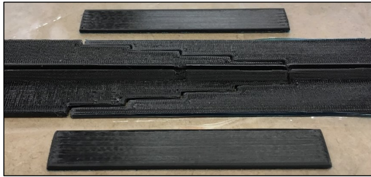
Figure 6.20. Carbon fibre (CF) composite strips for additional reinforcement of the scarf joints on the composite spar flanges.
