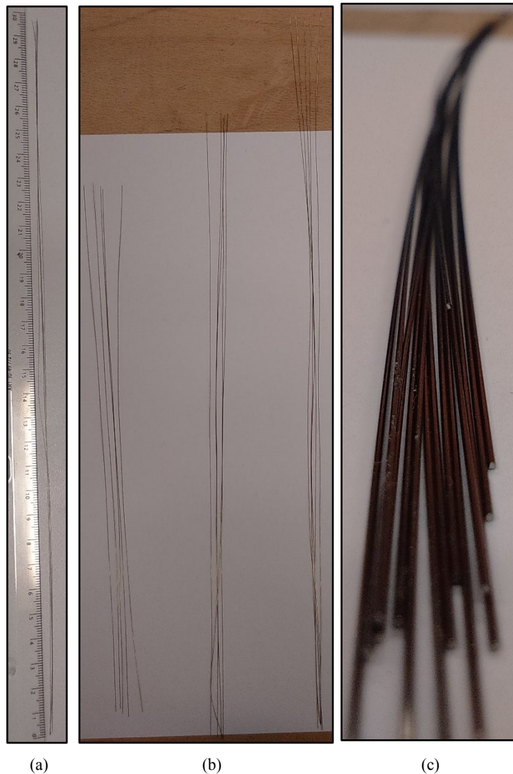
Figure 3.6. Shape memory alloy (SMA) wires with diameter of (a) 0.1 mm, (b) 0.2 mm and (c) 0.5 mm.
