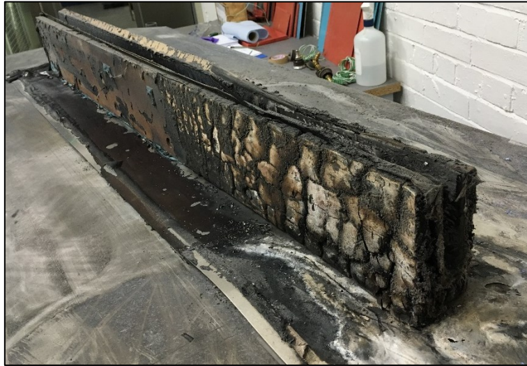
Figure F3. The burned CF composite prepregs and wood female mould on the first trial of manufacture of the CF composite D-nose skin.
