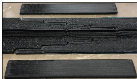
Figure 6.21. Evolution of the design and manufacturing iterations of the 3D-printed CF composite spar flanges.
