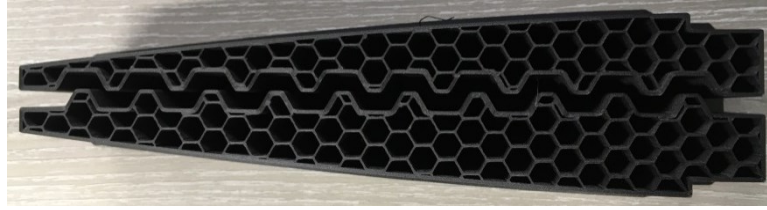
Figure 5.72. An example of a cellular honeycomb structure to form smooth upper and lower aerofoil surfaces.
