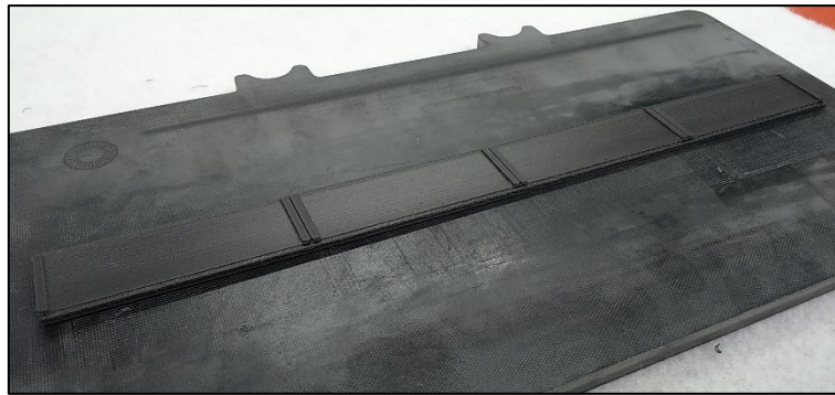
Figure 6.22. Initial design of 3D-printed CF composite spar web.
