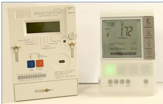
Figure 2.2: the Landis and Gyr E470 with in-home display.
