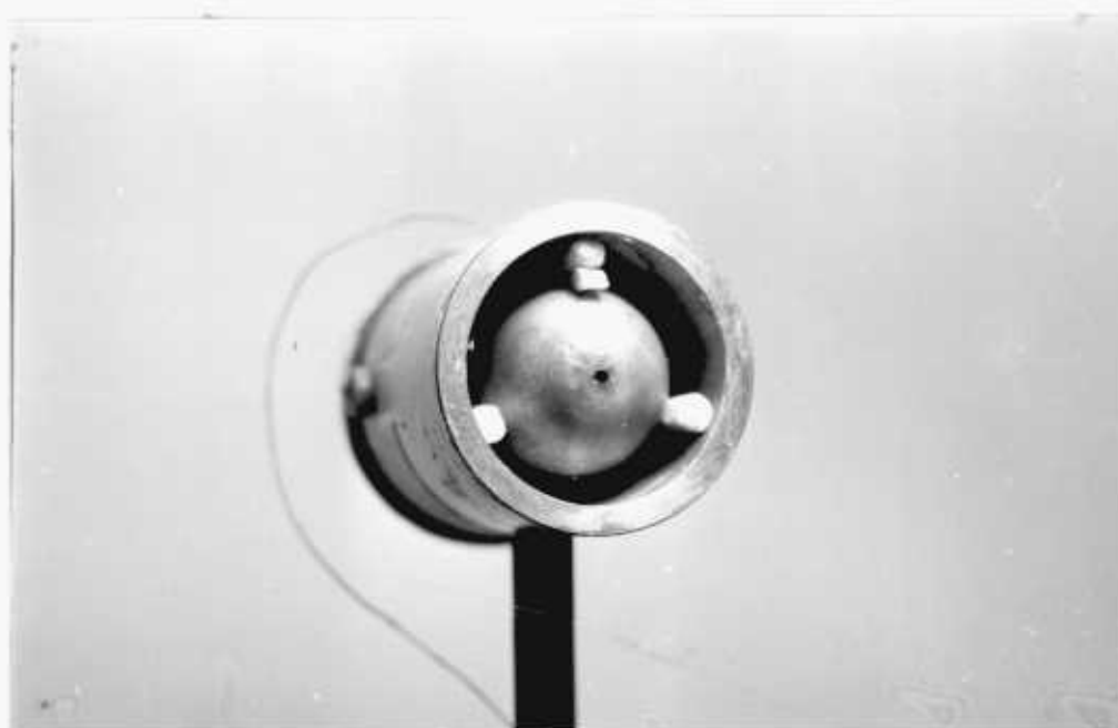
Fig. 2.4 Beam energy calorimeter in polished metal cavity
