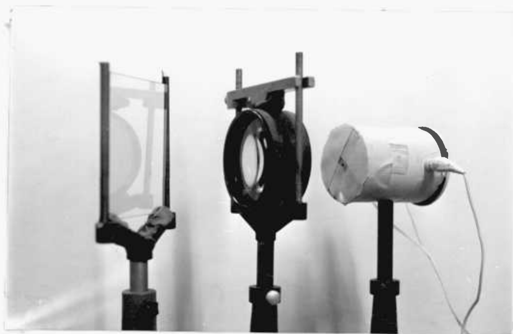
Fig. 2.5 Beam splitter, condensing lens and beam energy calorimeter
